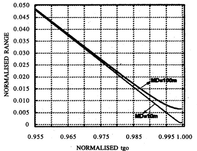
Figure 12. Missile-to-target range
