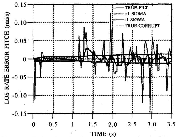
Figure 9. Estimation of seeker state using an adaptive Kalman filter. The LOS rate error pitch (filtered and true).
