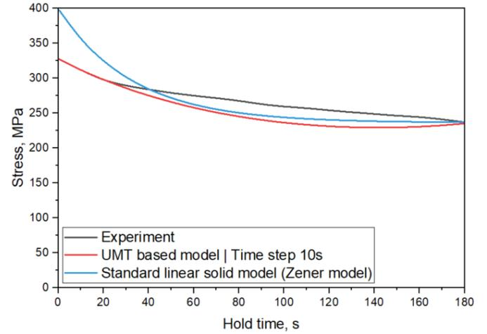
**Figure 4.** Comparison of the stress relaxation experimental data and predicted values for DZ445 material at  $900\text{ }^\circ\text{C}$ ,  $1.6\%$  strain range, and 3 minutes hold time with 10s time step size. UMT-based simulation captures the stress relaxation behaviour, which can be easily validated with experiments.
