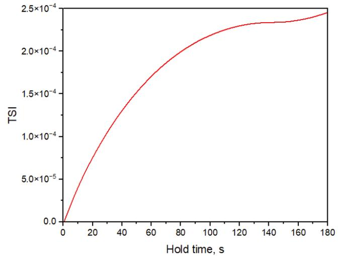
Figure 9. Development of TSI with hold time derived from UMT-based model for DZ445 material at 900 °C, 1.6 % strain range and 3 min. hold time with 10s time step size.
