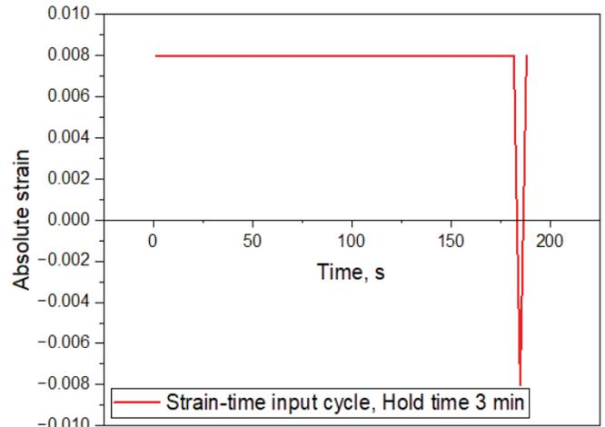
Figure 1. Input cycle of creep-fatigue interaction loading: Strain-time plot with 3 min hold time.
