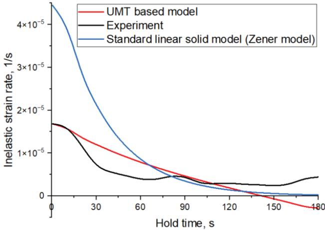
Figure 7. Comparison of modelling creep strain rate with experimental creep strain rate for DZ445 material subjected to creep-fatigue interaction loading at 900 °C, 1.6 % strain range, and 3 min. hold time with 10s time step.
