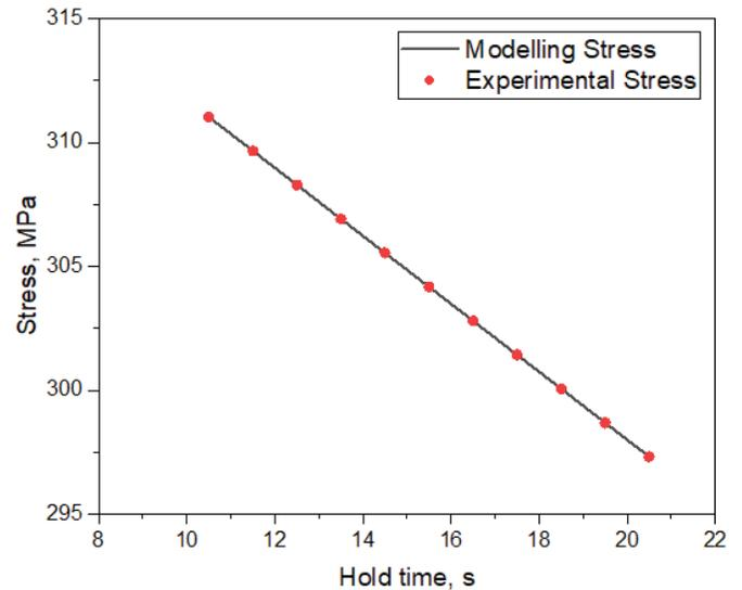
**Figure 3. After optimization, an agreement between the proposed model and experimental values for an initial time interval of 10 sec.**
