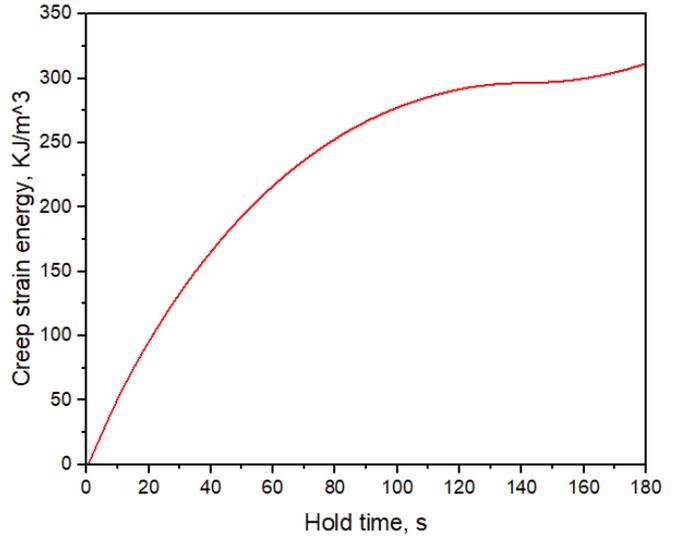
Figure 8. Variation of creep strain energy with hold time derived from UMT-based model for DZ445 material subjected to creep-fatigue interaction loading at 900 °C, 1.6 % strain range, and 3 min. hold time with 10s time step.
