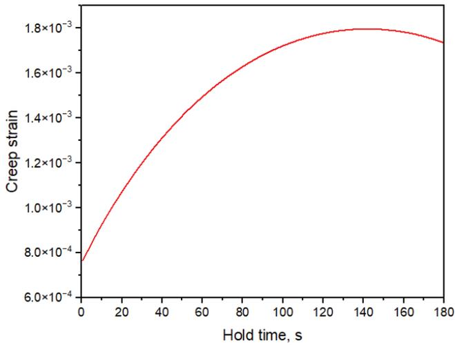
Figure 6. Variation of creep strain with hold time derived from UMT-based model for DZ445 material subjected to creep-fatigue interaction loading at 900 °C, 1.6 % strain range, and 3 min. hold time with 10s time step
