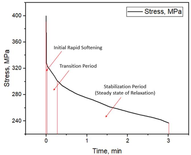
Figure 2. Stress relaxation experimental data<sup>12</sup> of DZ445 subjected to creep-fatigue interaction loading with 3 min hold time and 1.6 % strain range at 900 °C.
