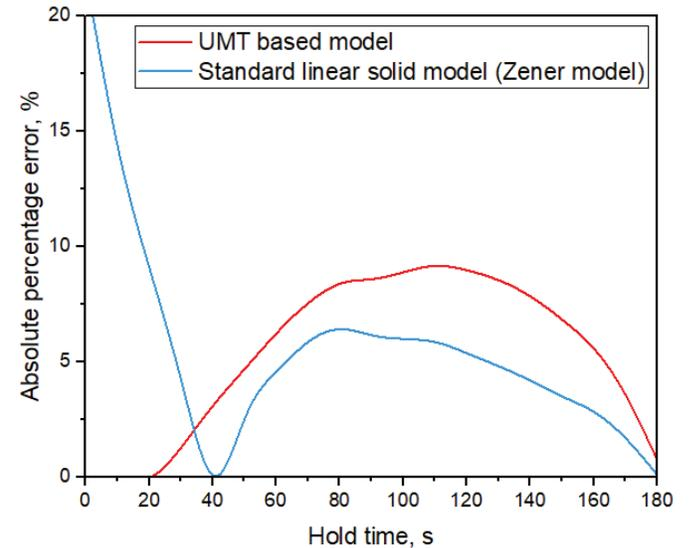
**Figure 5.** Absolute percentage error calculated during the hold time, which consistently remains less than  $10\%$  for proposed UMT-based model.
