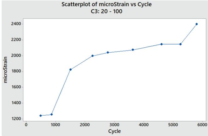
Figure 12. Micro-strain vs number of cycles plot for C3: 20 – 100.
