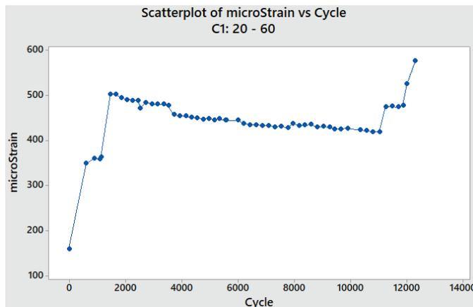
Figure 8. Micro-strain vs. number of cycles plot for C1: 20 - 60.
