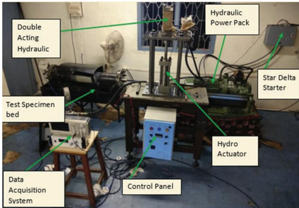
Figure 4. Cyclic Loading Setup.
