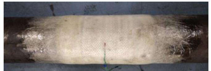
Figure 11. Failed specimen with 80 % wall loss due to cyclic loading of 20 bar to 80 bar.
