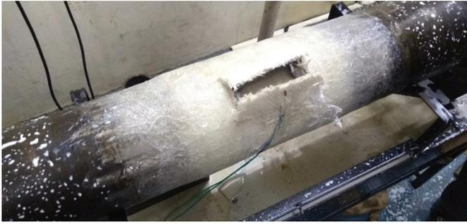
Figure 7. Failed specimen with 80 % wall loss.
