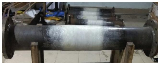
Figure 2. Test pipe specimens repaired with CSM + WRM (2+4) composite wrap.
