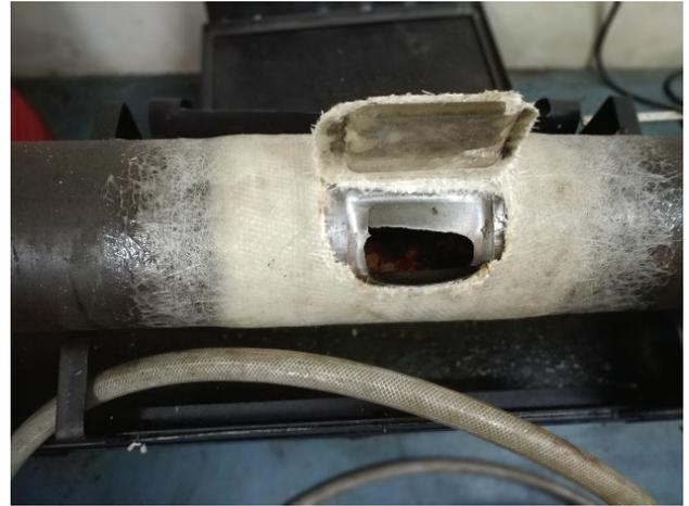
Figure 9. Failed specimen with 80 % wall loss after cyclic loading of 20 bar to 60 bar.
