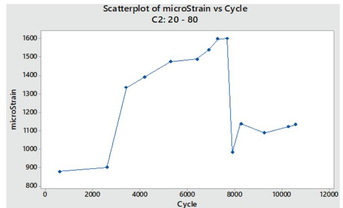
Figure 10. Micro-strain vs number of cycles plot for C2: 20 - 80.
