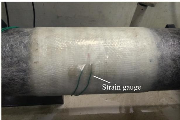
**Figure 5. Strain gauge mounted in the circumferential direction over the defect.**
