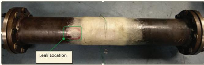
Figure 13. Failed specimen with 80 % wall loss due to cyclic loading of 20 bar to 100 bar.
