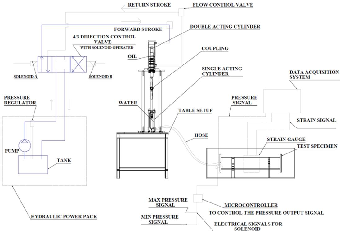
Figure 3. Schematic Layout of Cyclic Loading Setup.
