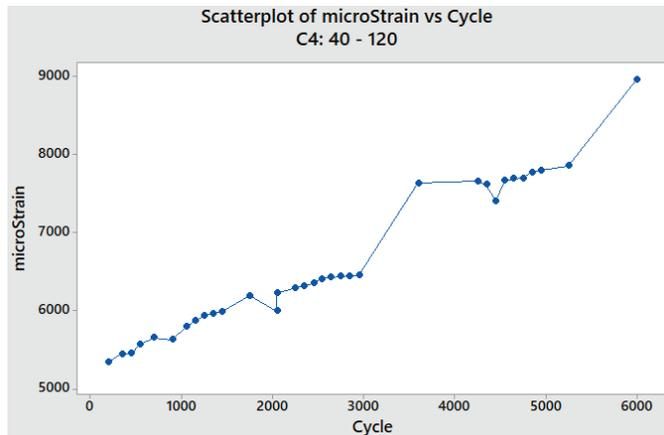
Figure 14. Micro-strain vs number of cycles plot for C4: 40 – 120.
