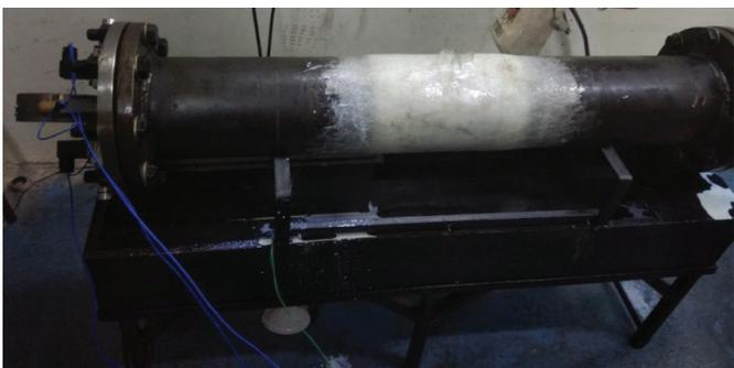
Figure 15. Failed specimen with 80 % wall loss due to cyclic loading of 40 bar to 120 bar.
