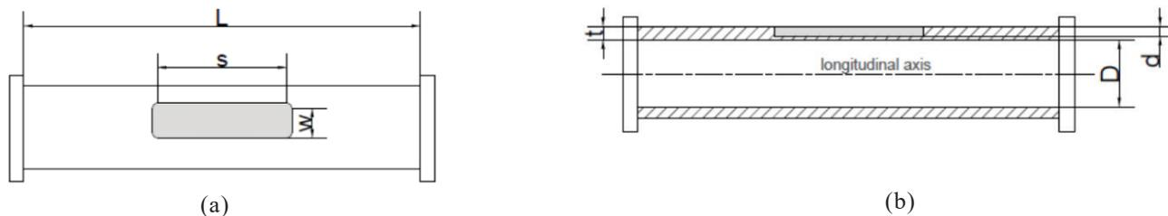
Figure 1. Pipe specimen with non-leaking wall loss defect (a) Top view (b) Front cut-sectional view.
