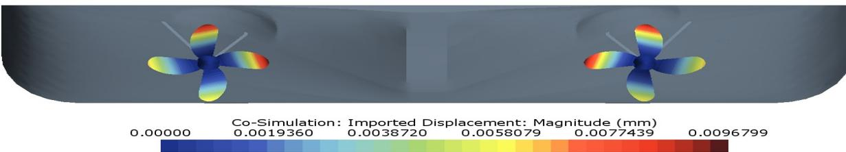
Figure 10. CFRP displacement for Sequence B.
