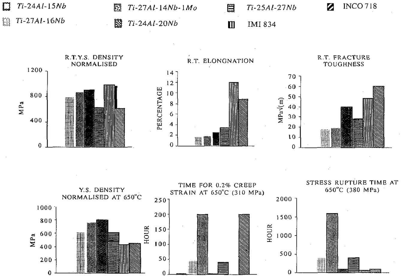
Figure 10. Comparison of  $Ti_xAl/Ti_yAl Nb$  alloys with IMI 834 and INCO 718
