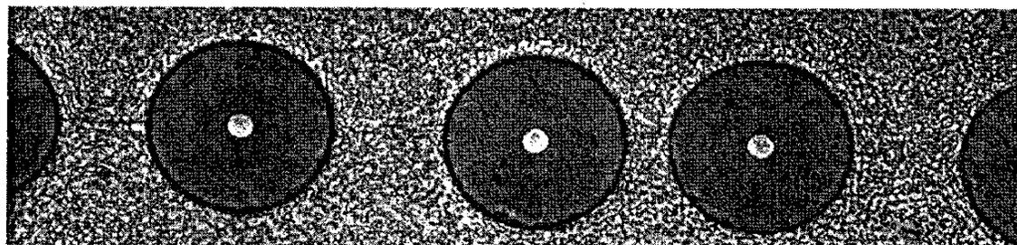
Figure 14. *Ti-22Al-25Nb/SiC* composite produced by fibre foil method utilising foil developed at the DMRL
