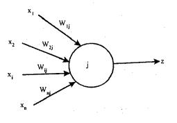
Figure 2. Single processing unit
