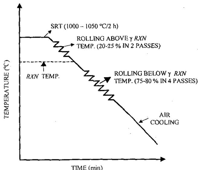
Figure 6. The optimised thermomechanically-controlled processing schedule.
