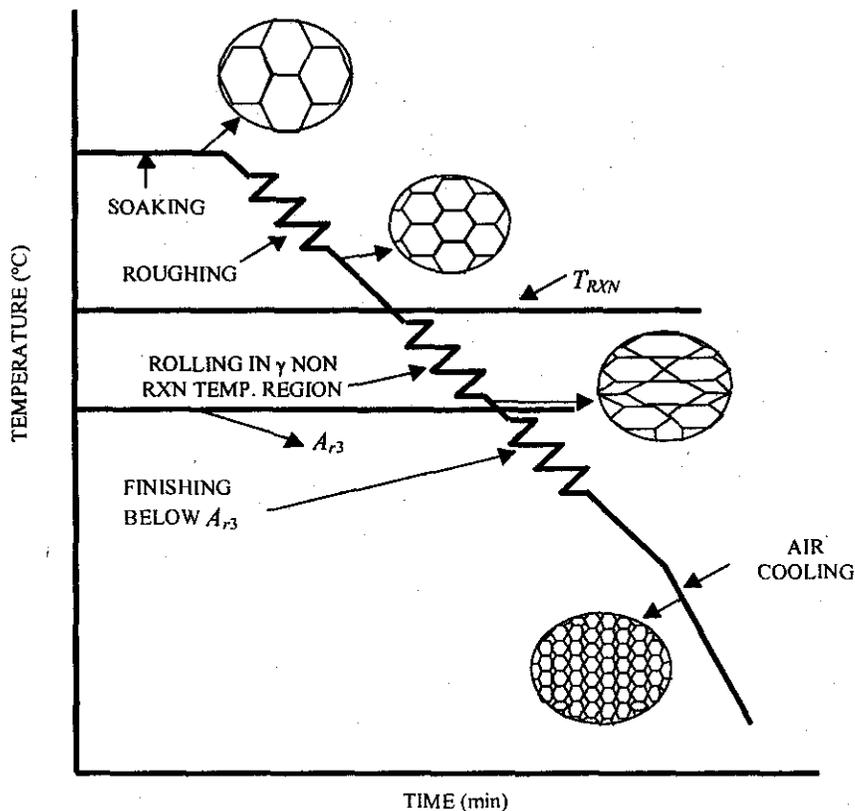
Figure 4. Typical thermomechanically-controlled processing schedule
