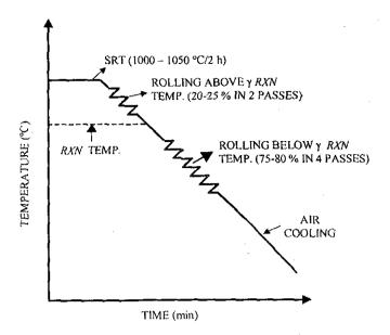
Figure 6. The optimised thermomechanically-controlled processing schedule.
