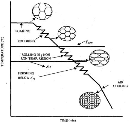
Figure 4. Typical thermomechanically-controlled processing schedule
