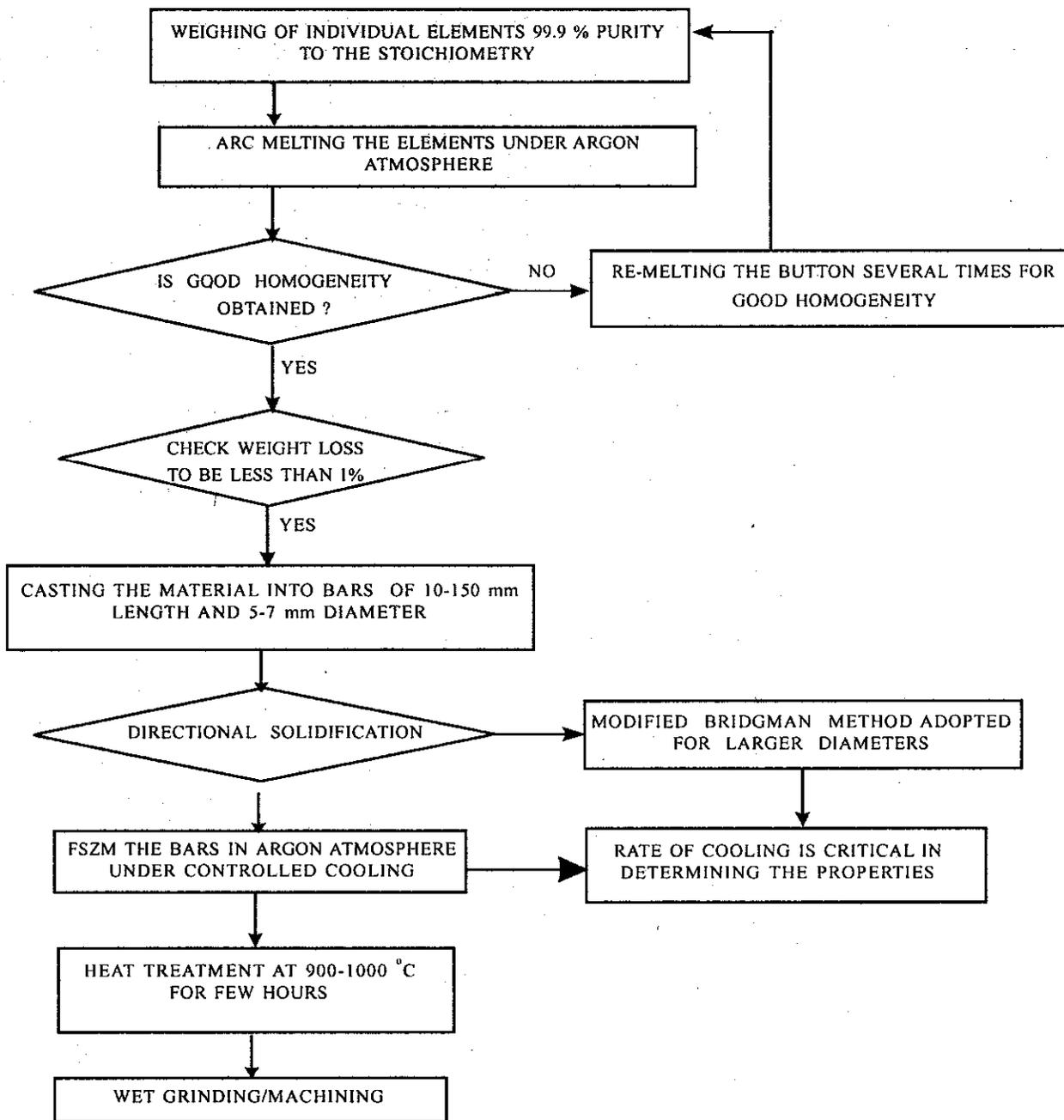
Figure 2. Flow chart for material preparation
