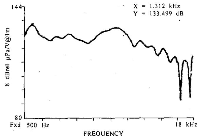
Figure 5. Transmitting voltage response of the transducer
