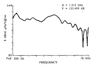
Figure 5. Transmitting voltage response of the transducer
