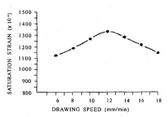
Figure 1. Variation in magnetostriction values versus rate of cooling.
