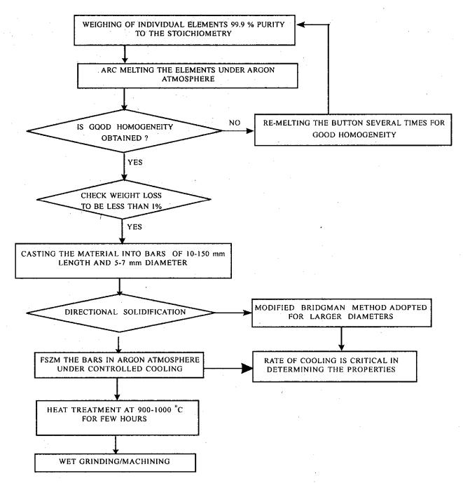
Figure 2. Flow chart for material preparation
