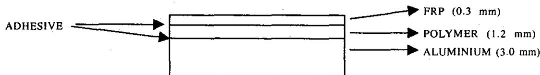
Figure 2. Construction of a constrained-layer damping system
