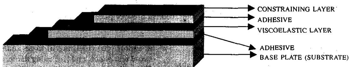
Figure 1. Schematic diagram of a constrained-layer damping system
