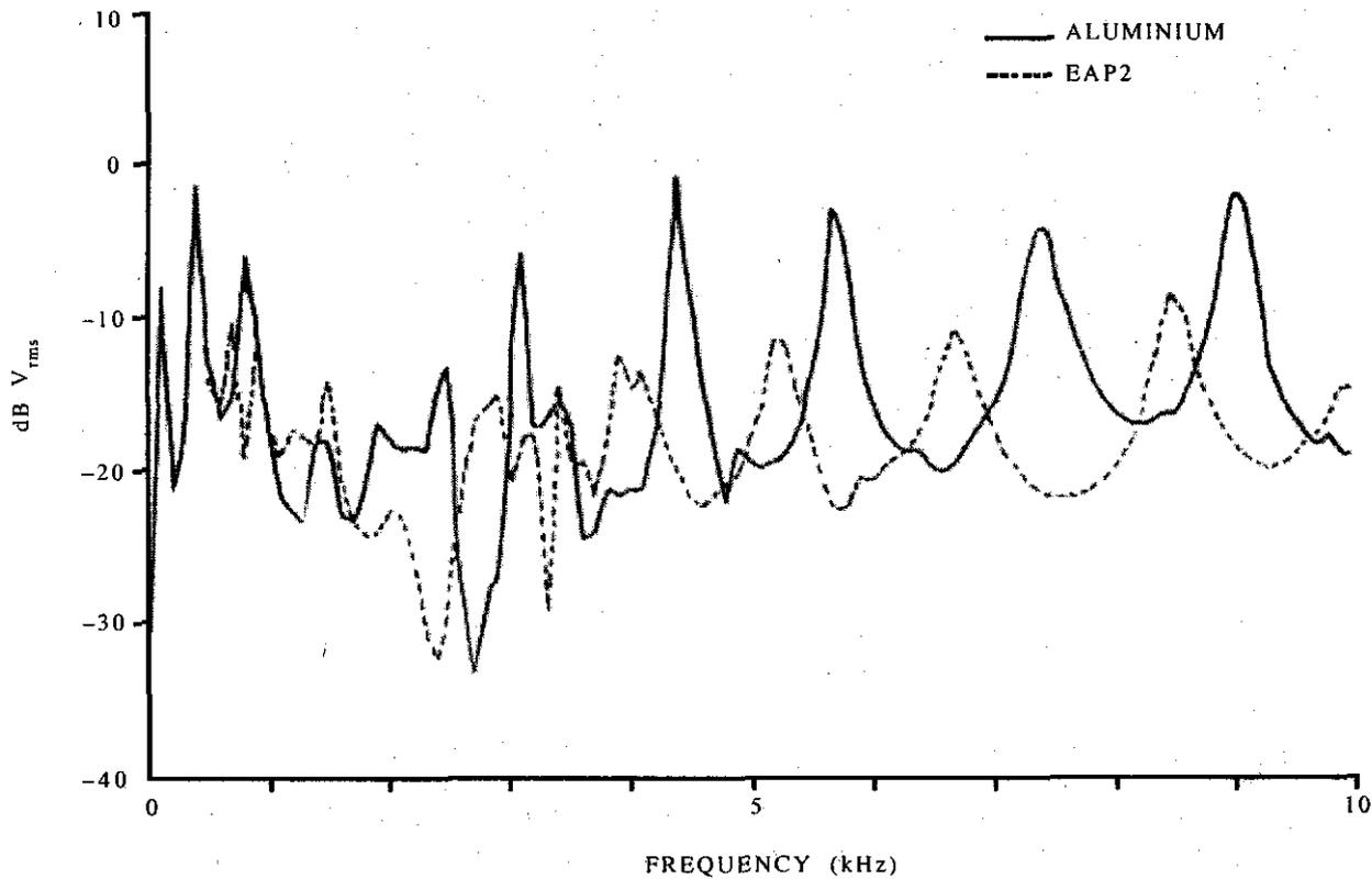
Figure 6. Plot of CLD acceleration data of a bare aluminium plate and a CLD system containing EAP2 as the damping layer
