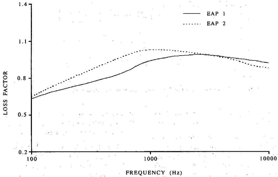
Figure 4. Dynamic mechanical properties of the two polymer compositions EAP1 and EAP2
