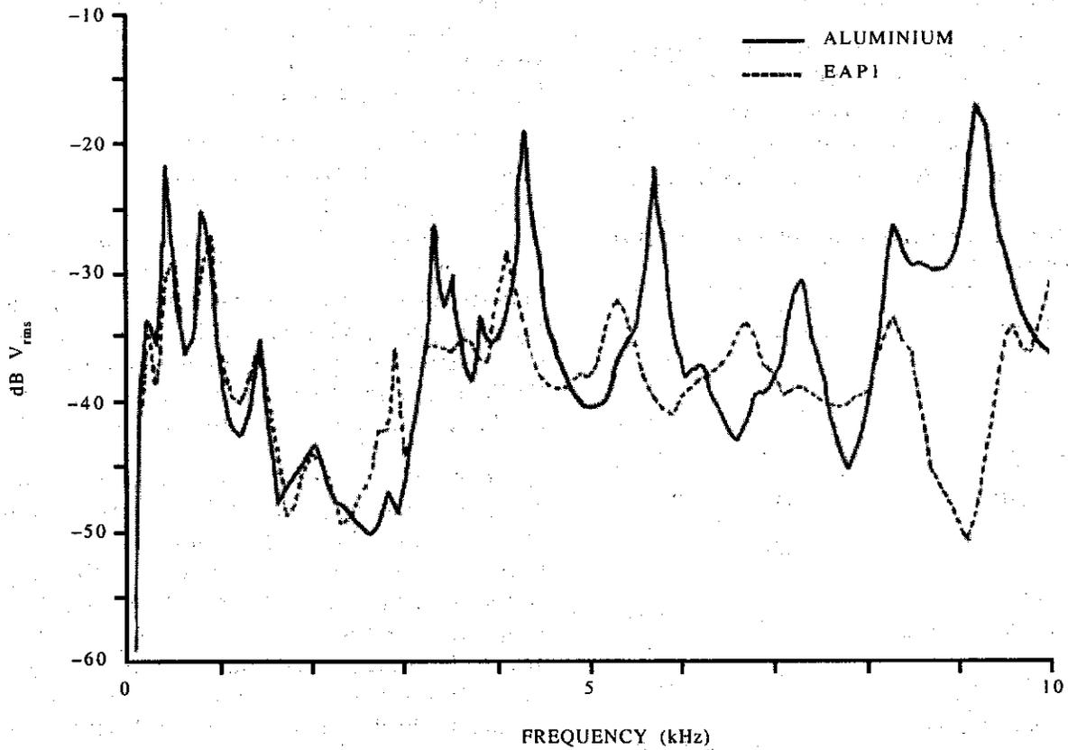
Figure 5. Plot of CLD acceleration data of a bare aluminium plate and a CLD system containing EAP1 as the damping layer
