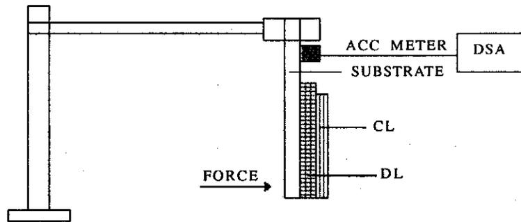
Figure 3. Experimental setup for measurement of vibration response
