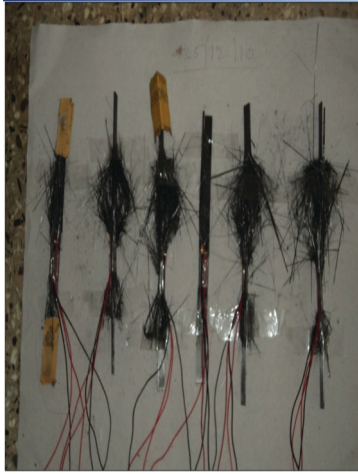
Figure 3. Failure modes of test results of composite specimens ( V_f = 60\% ).
