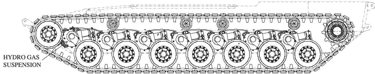
Figure 1. Running gear for a typical tracked vehicle.
