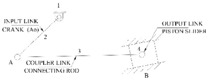
Figure 4. Four-bar mechanism of hydro gas suspension.
