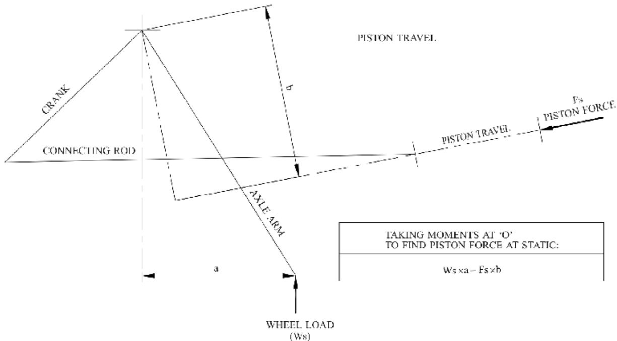
Figure 5. Kinematic arrangement of a typical hydro gas suspension.
