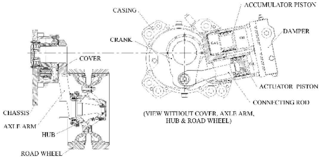
Figure 3. Internal arrangement of a typical hydro gas suspension system.
