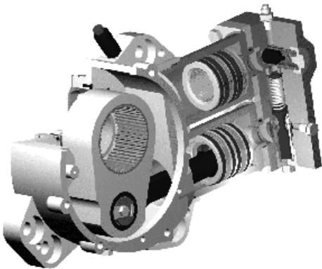
Figure 2. Cut-section model of a typical hydro gas suspension.
