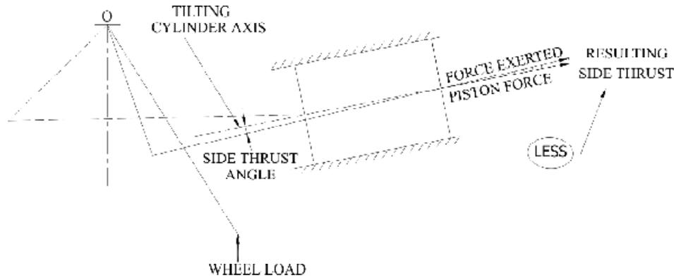
Figure 8. Effect of side thrust with cylinder offset and reorientation of cylinder.
