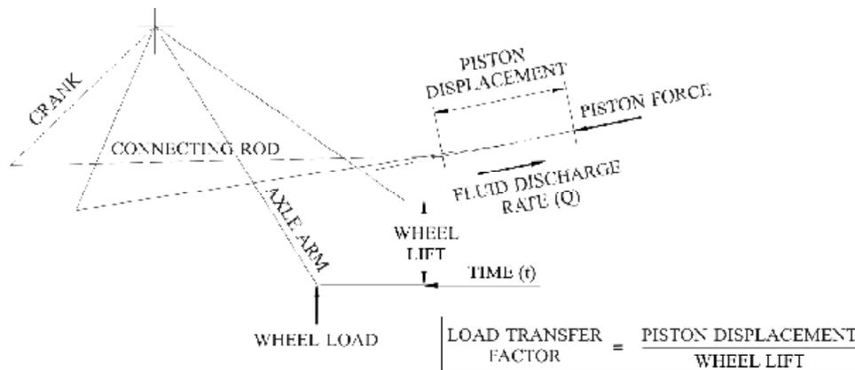
Figure 9. Load transfer factor for a given wheel lift.
