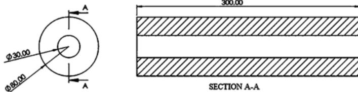
Figure 3. Straight fuel geometry.
