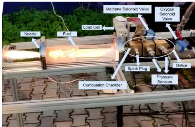
**Figure 12. Appearance of the experimental equipment used in the first set of experiments.**
