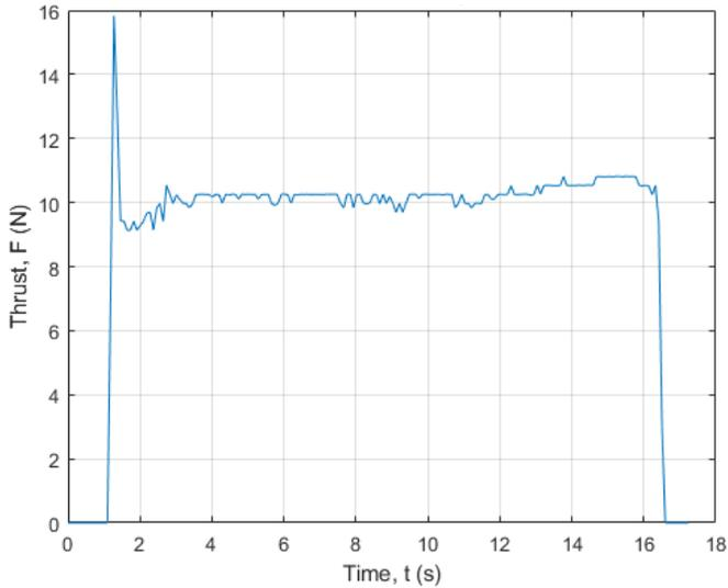
Figure 14. Thrust-time graph obtained as a result of the experiment (Straight fuel).
