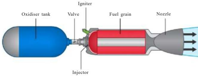
Figure 1. A typical configuration of a hybrid rocket engine<sup>7</sup>.
