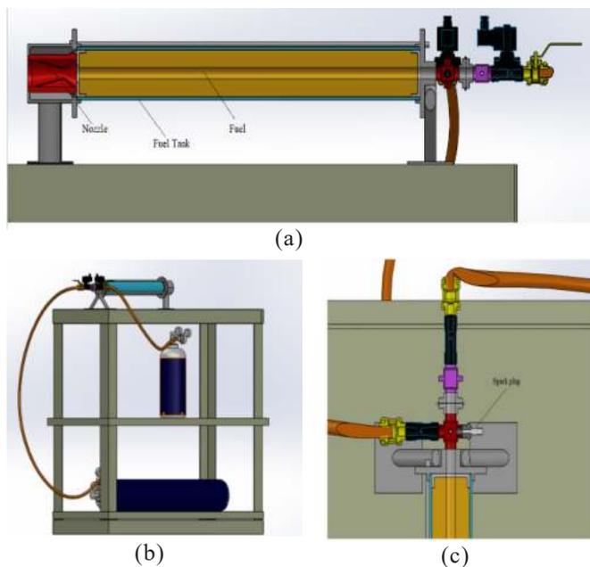
Figure 9. Computer aided design of (a) Combustion chamber, (b) Oxygen and methane cylinder, and (c) Spark plug and ignition system.
