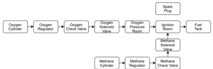
Figure 8. Assembly connection diagram.
