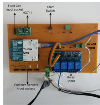
Figure 11. (a) Electronic circuit conceptual design, and (b) Electronic system on perforated copper plate.
