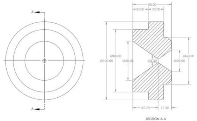
Figure 7. Converging-diverging nozzle dimensions.
