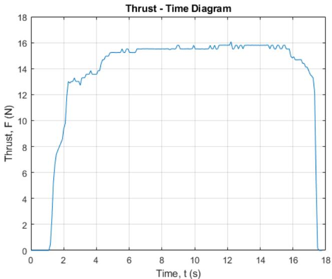
Figure 15. Thrust-time graph obtained as a result of the experiment (Square grooved fuel).
