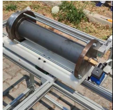
Figure 10. Final state of the experiment system (engine, oxygen inlet and load cell).
