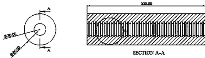
Figure 4. Square grooved fuel geometry.
