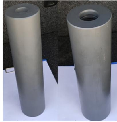
Figure 5. Straight and square grooved fuels used in the experiment.
