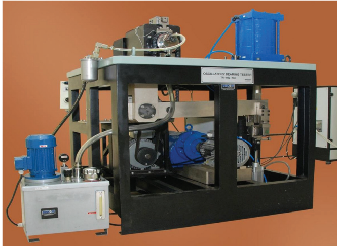
Figure 1. Oscillatory bearing test rig at CSIR-National Aerospace Laboratories.
