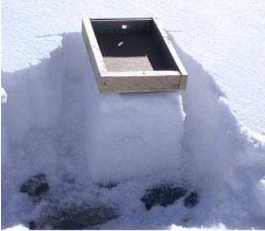
Figure 3. Wooden block placed over the snow column.
