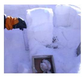
Figure 6. A column failed after few steps of loading.
