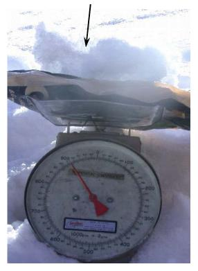
Figure 1. A snow block over the weighing machine for loading the snow columns but snow grains disintegrated in large amount during the preparation and weighing of snow block.
