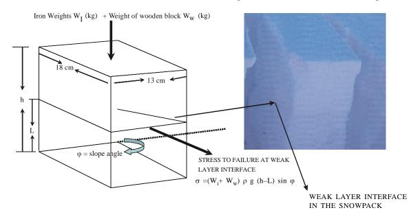
Figure 7. Schematic diagram of the test (showing stress to failure at weak layer interface, at a depth of (h-L) from snow surface).
