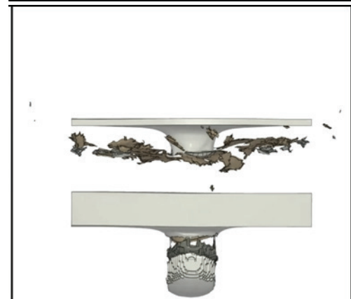
Figure 5. Bulge caused on the single high-hardness armour plate of Configuration 1 and Plugging failure observed in high-hardness armour plate of Configuration 2.
