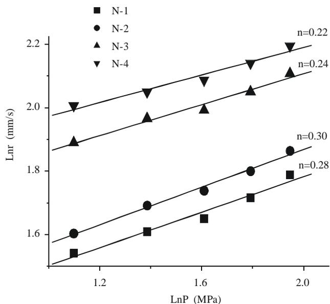
Figure 1. Burning rate and pressure exponent characteristics for propellants N-0~N-4.
