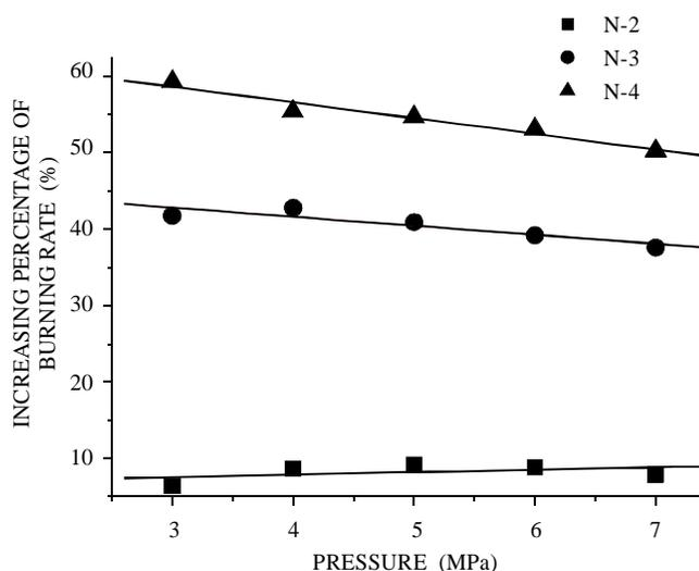
Figure 2. Increasing percentage of burning rate for propellants N-2~N-4 compared with propellant N-1.
