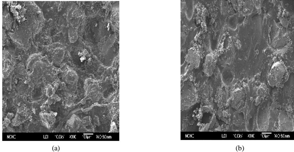
Figure 5. SEM of (a) N-1 propellant surface before combustion, and (b) N-4 propellant surface before combustion.
