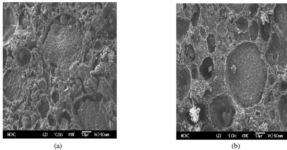
Figure 6. SEM of the burning surface of (a) N-1 propellant quenched at 1 MPa, and (b) N-4 propellant quenched at 1MPa.
