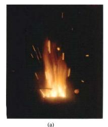
area of flame becomes large and uniform. The recorded particles burning trajectories show pronounced jetting phenomena. These could be caused by decomposition gas from the molten liquid and ejected through the oxide lobe. This phenomenon appears not to be obvious in N-1 propellant at 4.9 MPa.
