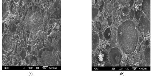
Figure 6. SEM of the burning surface of (a) N-1 propellant quenched at 1 MPa, and (b) N-4 propellant quenched at 1MPa.
