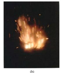
Figure 3. Flame images of N-1 propellant at (a) 0.49 MPa and (b) 4.9 MPa.
