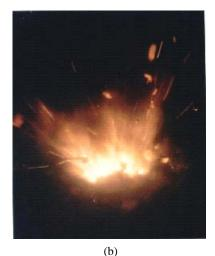
Figure 4. Flame images of N-4 propellant at (a) 0.49 MPa and (b) 4.9 MPa.
