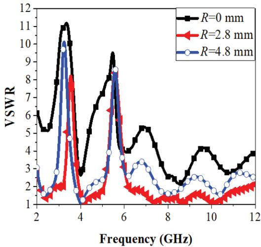
Figure 3. Impact of circular cavity radius on the impedance bandwidth of the VA.
