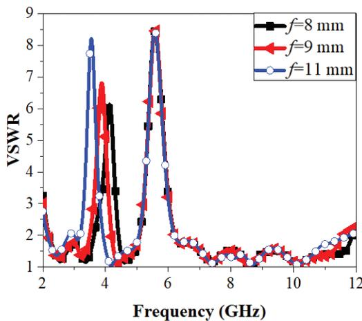
Figure 5. Impact of additional strip length on the impedance bandwidth of the VA.
