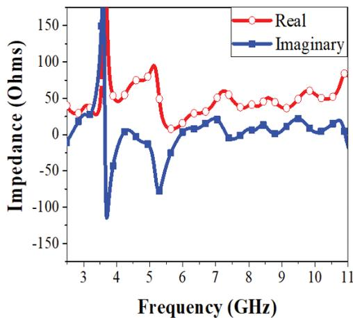
Figure 9. Impedance of the VA.
