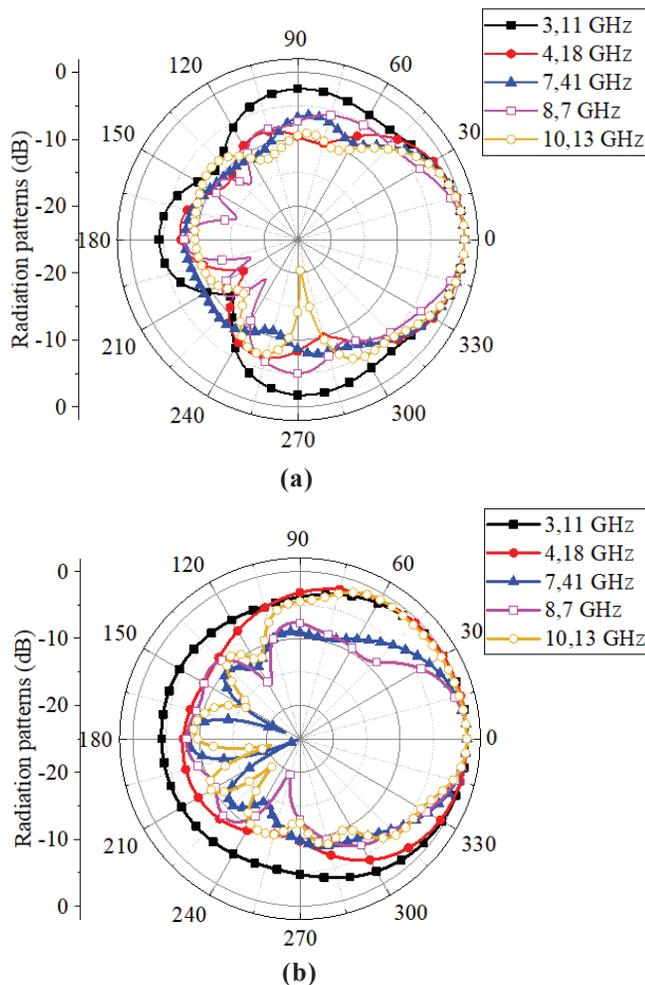
Figure 12. Normalised radiation patterns of the VA, (a) H-plane, and (b) E-plane.
