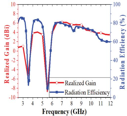
Figure 13. Realised gain and radiation efficiency of the presented VA.
