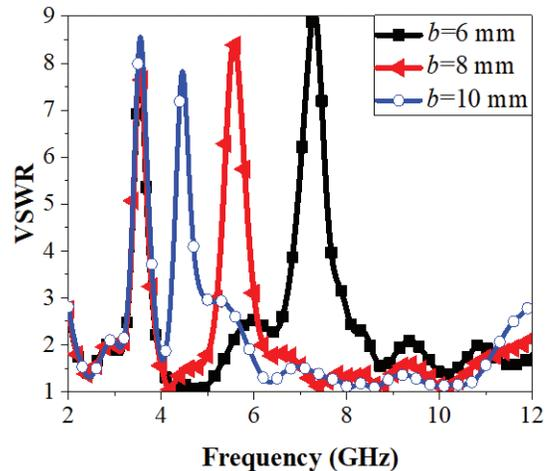
Figure 6. Impact of U-shaped slit length on the impedance bandwidth of the VA.
