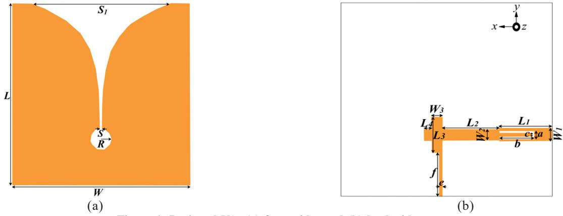
Figure 1. Designed VA; (a) front side; and (b) back side.
