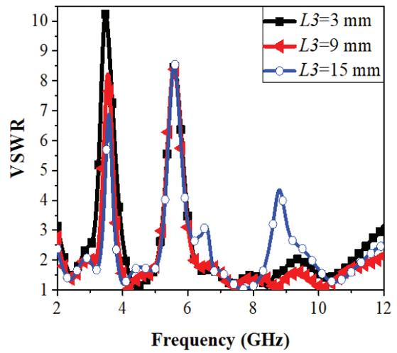
Figure 4. Impact of circular cross strip length on the impedance bandwidth of the VA.
