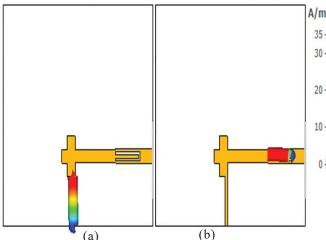
Figure 7. Current concentration on the surface of the VA at: (a) 3.55 GHz, and (b) 5.57 GHz.
