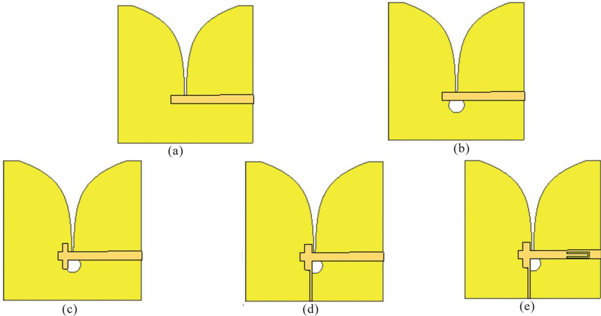
Figure 2. Structural development of the designed VA; (a) Antenna A; (b) Antenna B; (c) Antenna C; (d) Antenna D; and (e) Antenna E.
