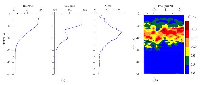
Figure 2. (a) Mean profiles of temperature, salinity, and Brunt-Vaisala frequency, N and (b) depth-time section of the stability parameter, E.
