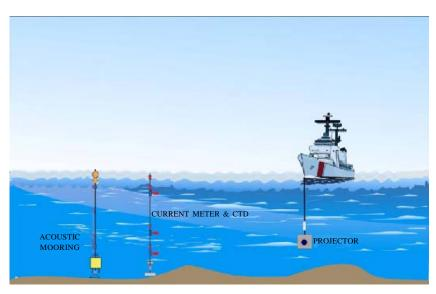
Figure 1. Experimental setup to study shallow water internal wave characteristic and their influence on acoustic propagation
