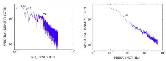
Figure 4. Spectral analysis of temperature data in the thermocline collected for (a) 15 h during 9-10 October 2002 and (b) 5 h on 8 October 2002. S1, S2, and S3 indicate peaks at ~6 h, ~3 h and near Brunt-vaisala frequency, ie, ~3 min, respectively.
