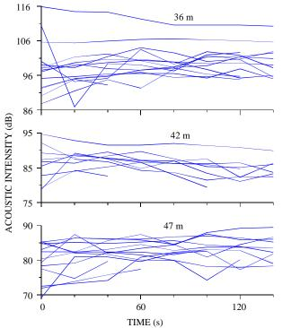
Figure 7. Composite plots of acoustic intensity for the entire 14 transmissions each of 2 min durations at every hour.
