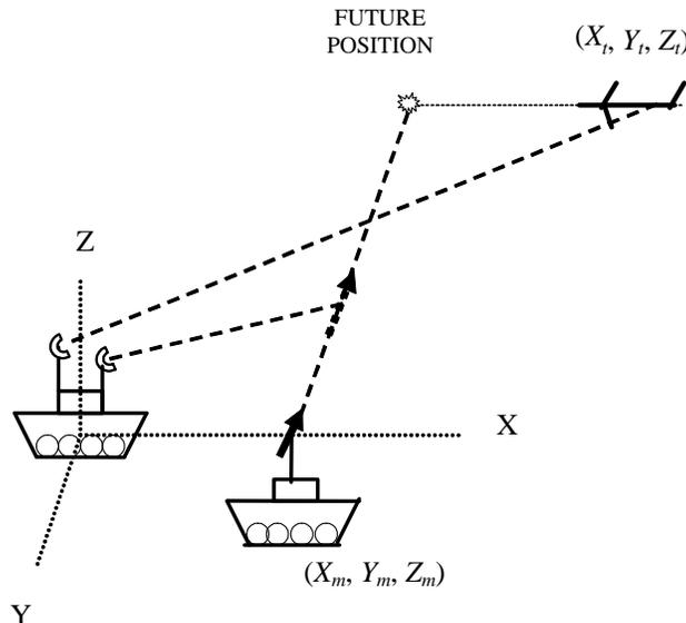
Figure 1. Two-platform system in the stabilised reference frame
