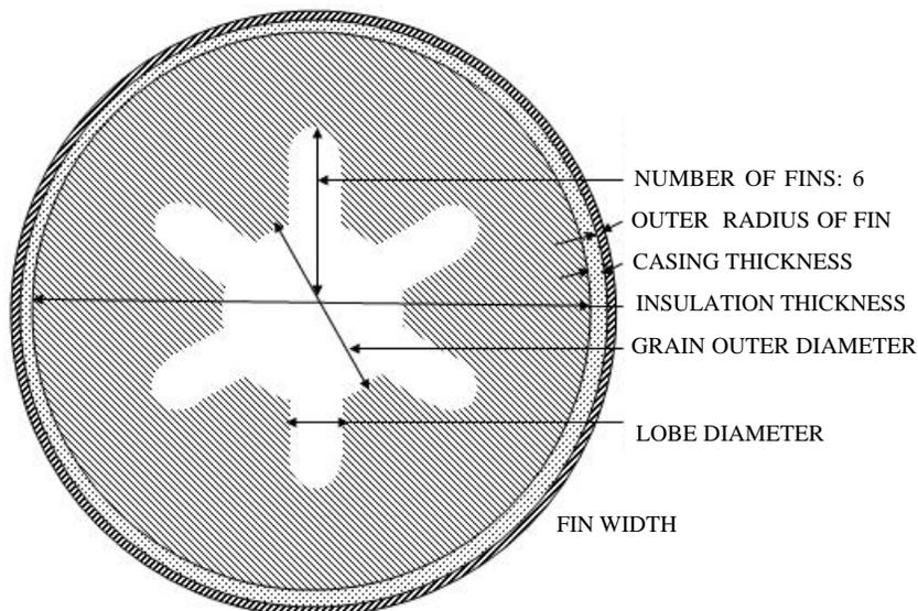
Figure 1. Geometrical parameters of finocyl-shaped port case-bonded propellant grain
