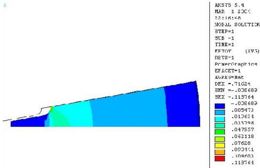
Figure 2. Strain plot for reference configuration under pressure loading
