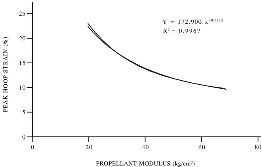
Figure 3. Variation of peak hoop strain with propellant modulus
