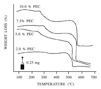
Figure 7. TG curves of *B-KNO*<sub>3</sub> system with various percentage of PEC atmospheric static air, HR 10 °C/min.
