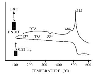
Figure 3. STA curves of *B-KNO*<sub>3</sub>–NC composition atmospheric static air, HR 10 °C/min.
