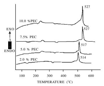
Figure 6. DTA curves of *B-KNO*<sub>3</sub> system with various percentage of PEC binder atmospheric static air, HR 10 °C/min.
