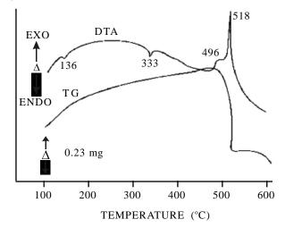
Figure 2. STA curves of *B-KNO*<sub>3</sub> (1:1) atmohpheric static air, HR 10 °C/min.
