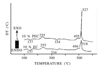
Figure 4. DTA curves of *B-KNO*<sub>33</sub> system with different binders, HR 10 °C/min.
