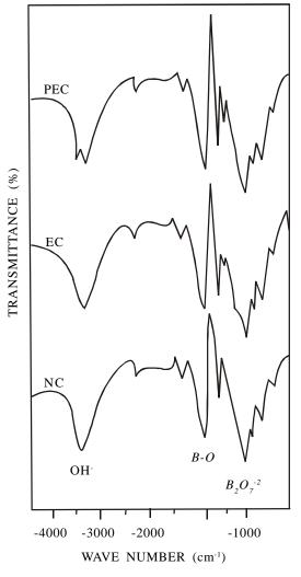
Figure 1. IR spectra of solid combustion products of *B-KNO*<sub>3</sub> system with different binders.
