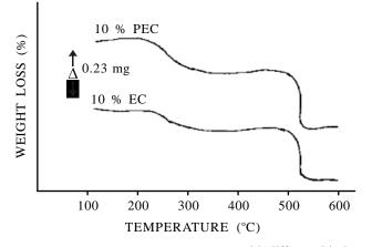
Figure 5. TG curves of *B-KNO*<sub>3</sub> system with different binders, HR 10 °C/min.
