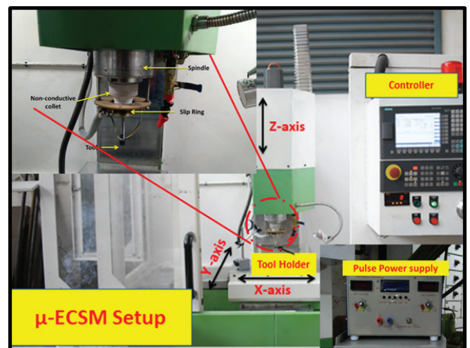
Figure 2. In-house developed \mu\text{-ECSM} setup.
