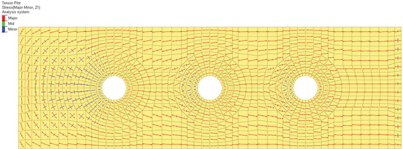
Figure 3. Directions of principle stress tensors.
