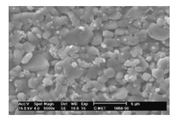
Figure 8. Microphotograph of MgO-doped alumina sintered at 1650 °C/90 min.
