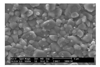
Figure 5. Microphotograph of  $MgO + SiO_2$ -doped alumina sintered at 1650 °C/90 min.
