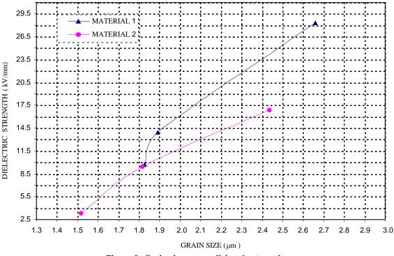
Figure 9. Grain size versus dielectric strength
