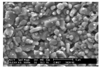
Figure 4. Microphotograph of  $MgO + SiO_2$ -doped alumina sintered at 1620 °C/90 min.
