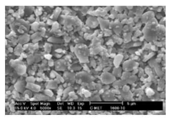
Figure 6. Microphotograph of *MgO*-doped alumina sintered at 1610 °C/10 min.
