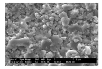
Figure 7. Microphotograph of MgO-doped alumina sintered at 1620 °C/90 min.
