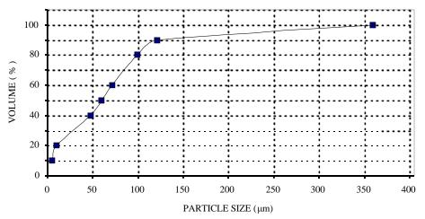
Figure 1. Particle size distribution of raw (unmilled) alumina powder
