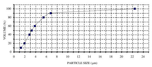
Figure 2. Particle size distribution of milled alumina powder
