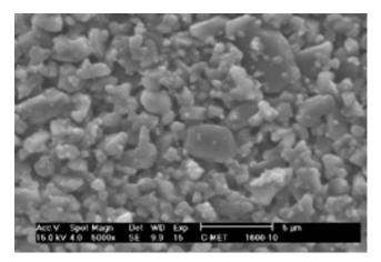
Figure 3. Microphotograph of  $MgO + SiO_2$ -doped alumina sintered at 1600 °C/10 min.
