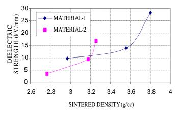
Figure 10. Sintered density versus dielectric strength
