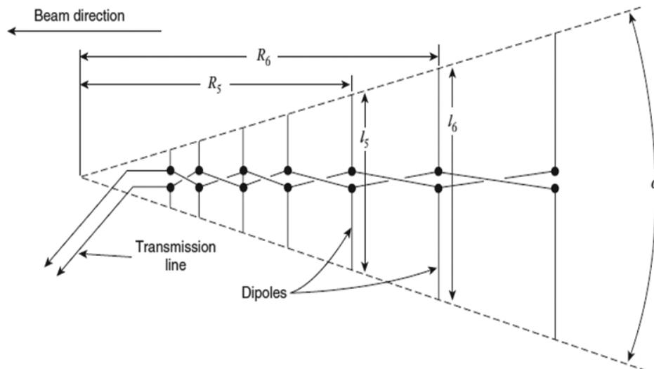
Figure 5. Log periodic dipole array.
