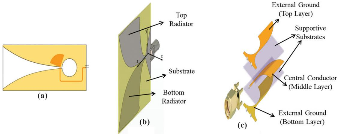
Figure 7. (a) Conventional coplanar vivaldi antenna; (b) CAVA; and (c) BAVA.
