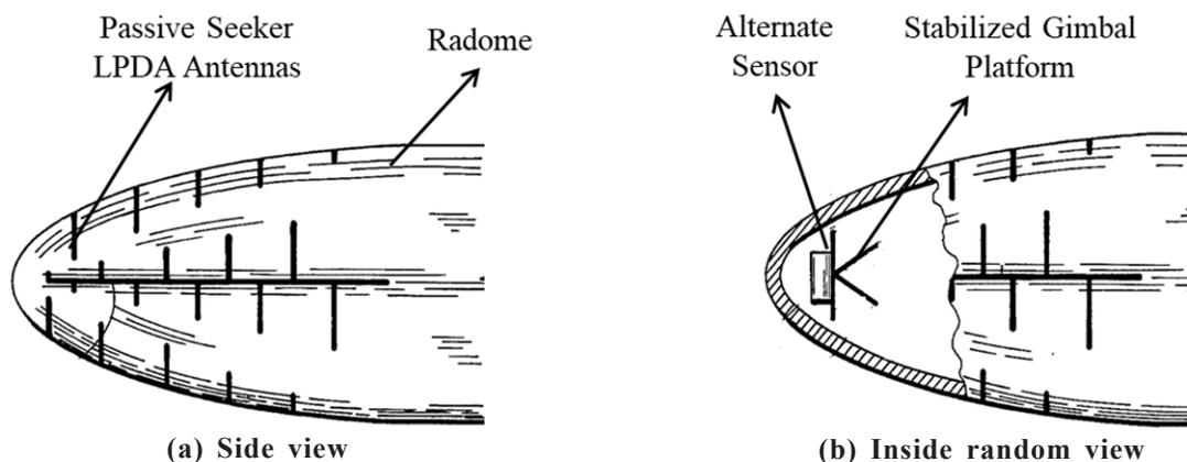
Figure 6. (a) Conformal LPDA23 for passive seeker application; and (b) Location of active/secondary terminal guidance sensor.
