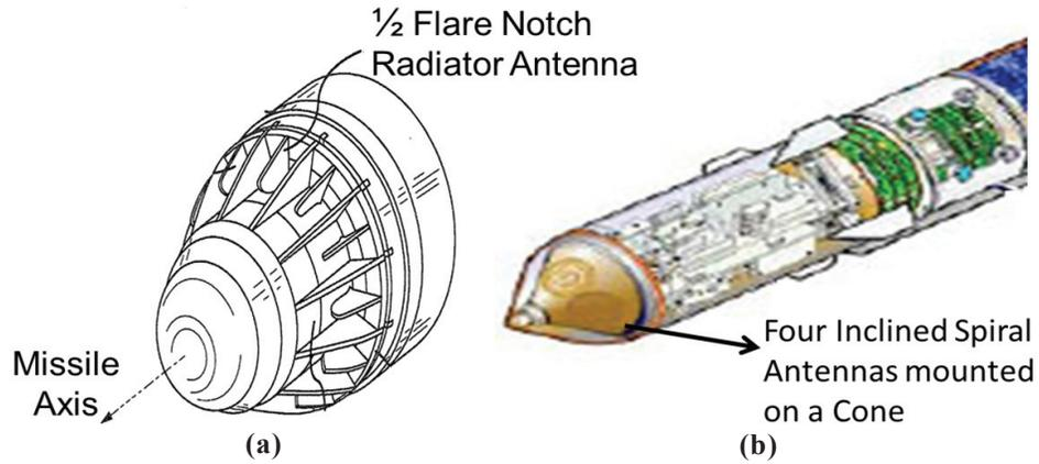
Figure 2. (a) Flush mounted notch radiator antenna<sup>8</sup>; (b) MAR-1<sup>9</sup>ARM with four flush mounted spiral antennas.
