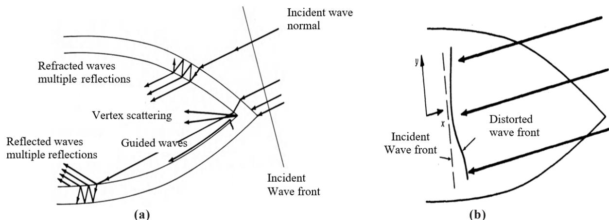
Figure 10. (a) Effect of missile radome<sup>57</sup> on incident wave; and (b) Distortion of EM wavefront by missile radome.
