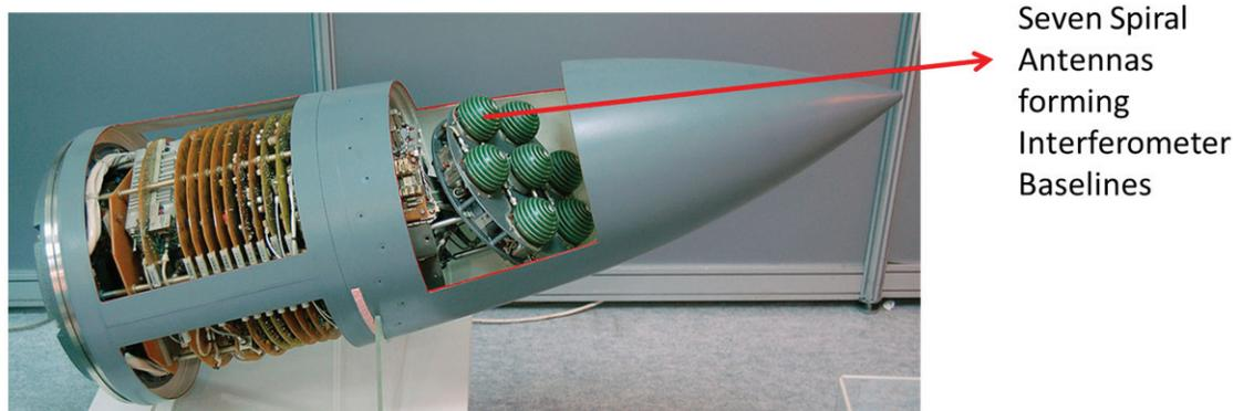
Figure 1. ARM Kh-31P<sup>7</sup> with spiral antennas concealed inside the radome.
