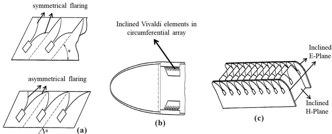
Figure 8. (a) Symmetrical flaring & asymmetrical flaring<sup>38</sup> of Vivaldi antenna; (b) Inclined vivaldi elements in circumferential array; and (c) Inclined E & H -Plane vivaldi.
