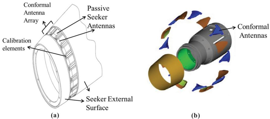
Figure 3. (a) Conformal antenna array on missile surface<sup>10</sup>; (b) Passive seeker of US AGM-88E ARM<sup>11</sup>with conformal antenna array.
