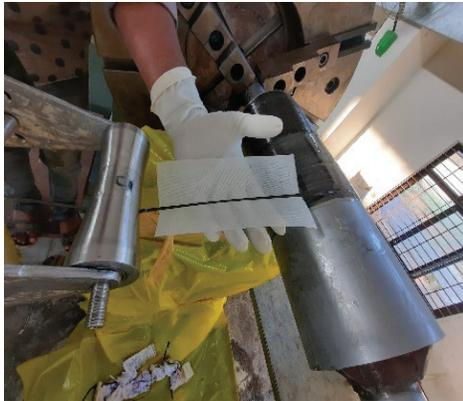
Figure 5. Impregnated fiber cutting.
