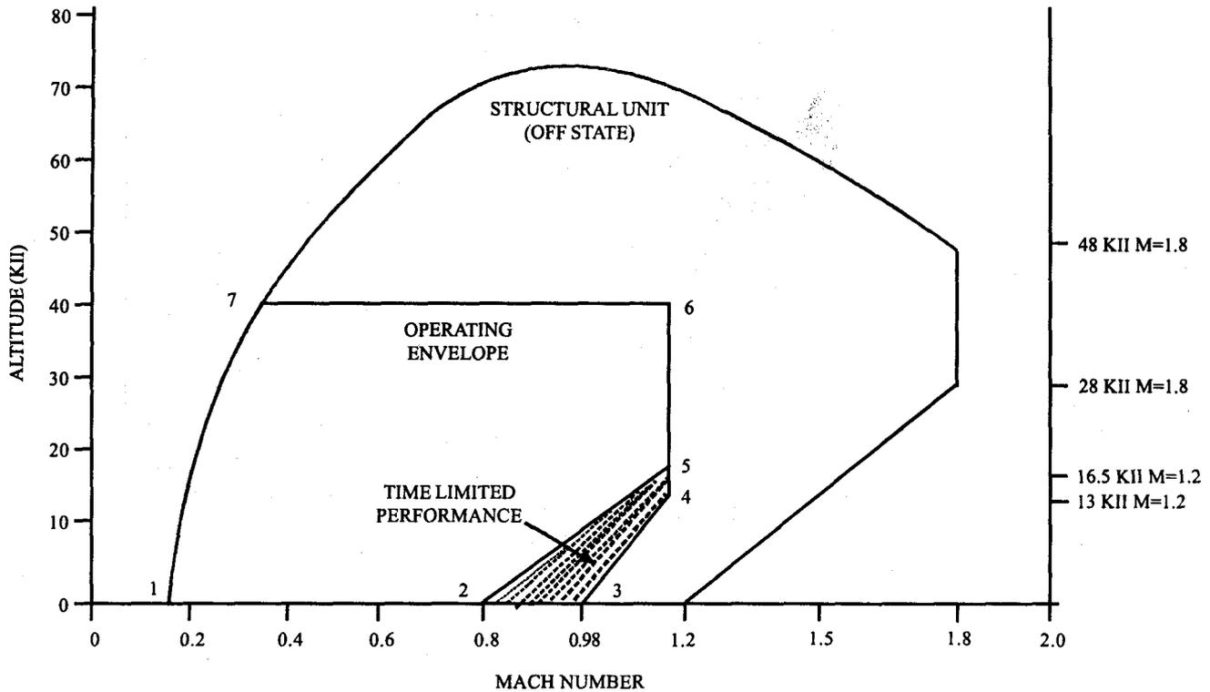
Figure 6. Pod's operational flight envelope for obtaining the expected pressure action on the radome
