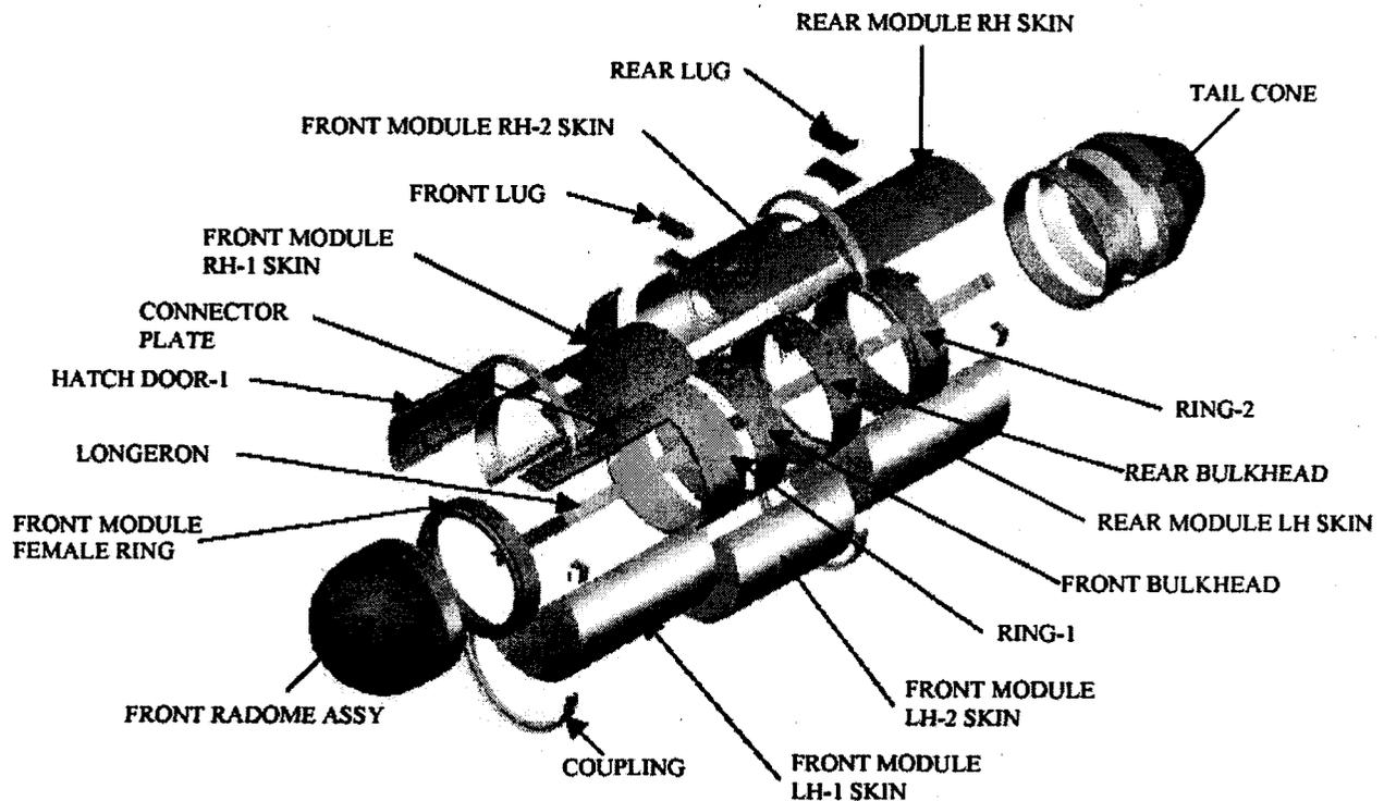
Figure 1. An exploded view of the pod
