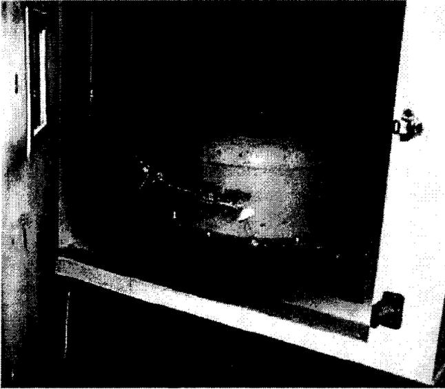
**Figure 8. Radome with the pressure cap in the high temperature test chamber.**
