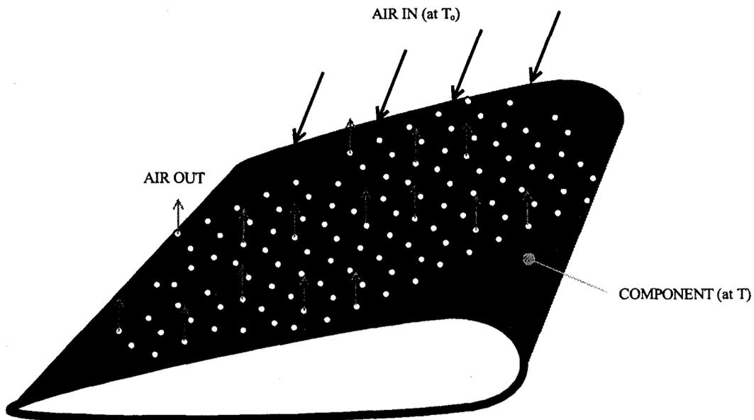
Figure 2. Fluid flow through cooling holes in a turbine component portion
