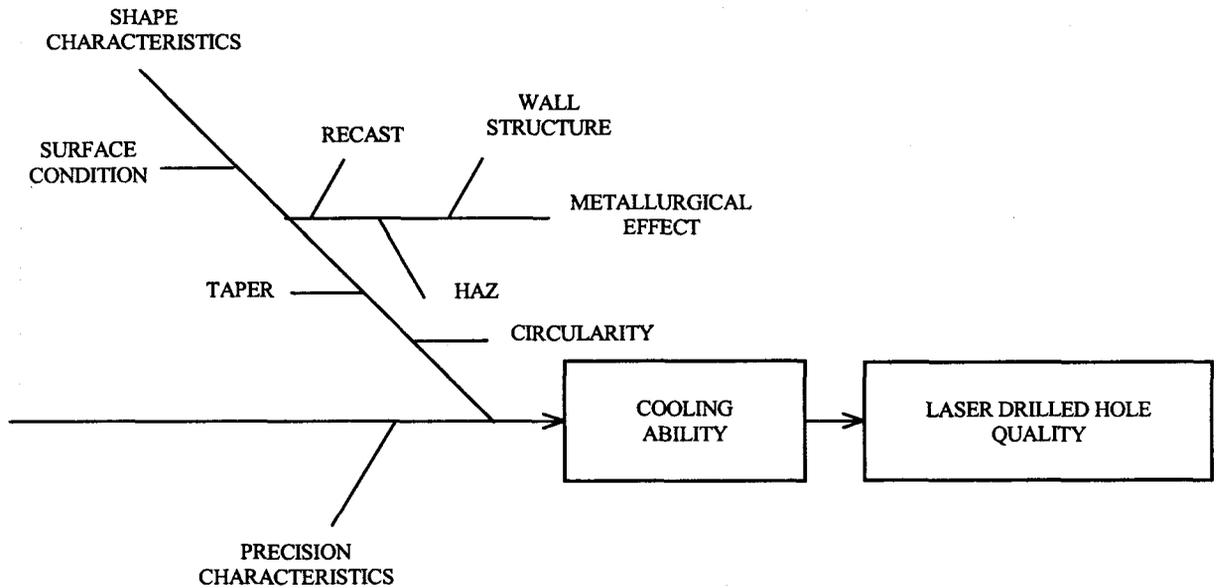
Figure 1. Percussion laser-drilled hole characteristics that affect its quality
