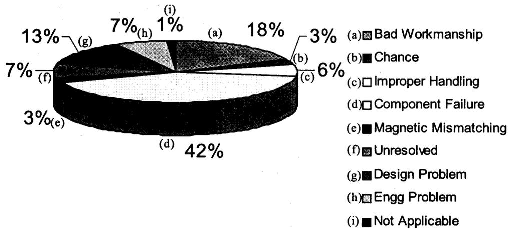
Figure 4. Causes of failures on Lakshya LRUs
