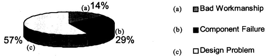
Figure 5. Causes of failure on Barco monitors (no. of failures: 7)
