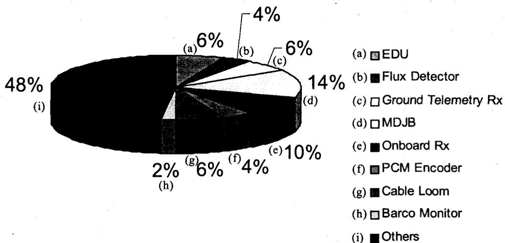
Figure 3. Failures on *Lakshya* LRUs (after delivery)
