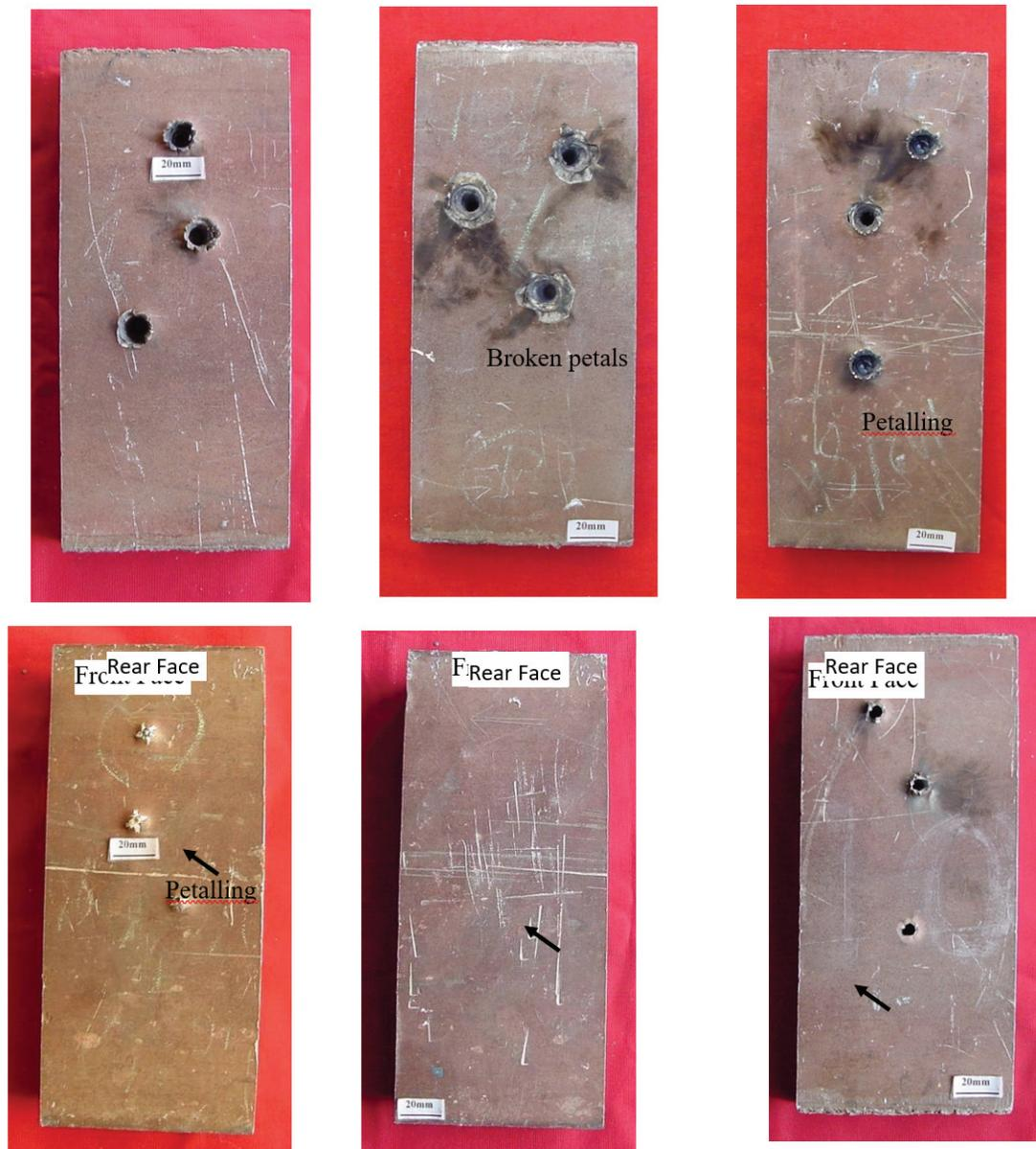
Figure 4. (a) Aged plates after ballistic impact.
