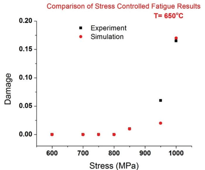
Figure 4. (b) Comparison of damage for experiment and simulation.
