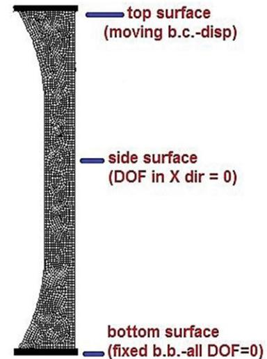
Figure 4. (a) FEM model of the specimen: mesh and boundary conditions.
