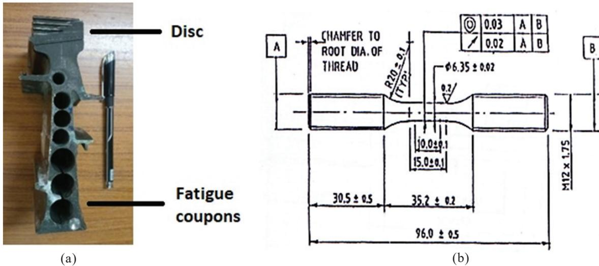
Figure 3. (a) Sample extraction from disc (b) LCF test sample (All dimensions are in mm).
