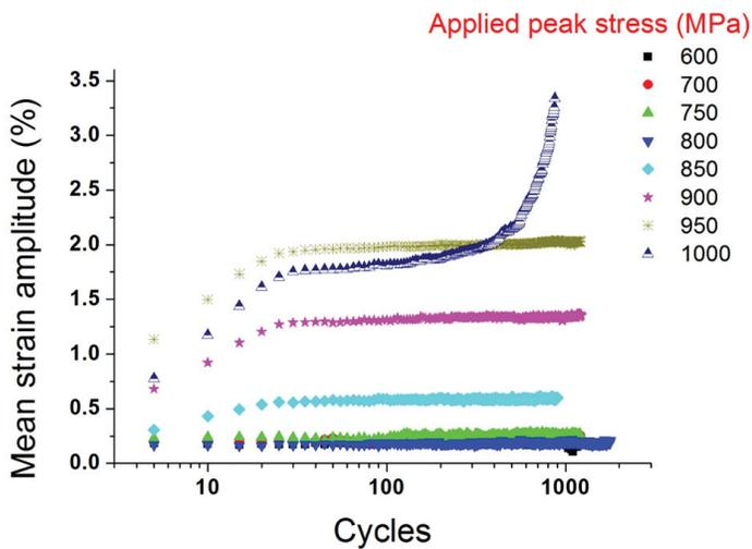
Figure 3. (c) Mean strain amplitude curves for samples tested under different applied peak stresses during incremental stress controlled fatigue tests at 650 °C.
