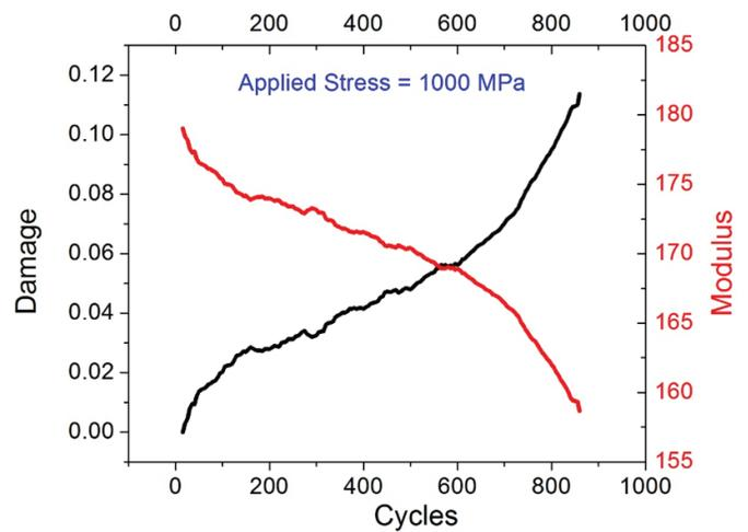
Figure 3. (e) Damage evolution curve for samples tested under 1000 MPa peak stresses during incremental stress controlled fatigue tests at 650 °C.
