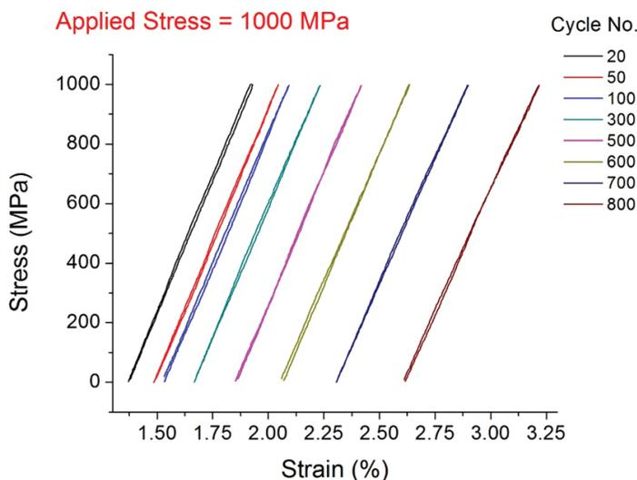
Figure 3. (d) Stress-Strain curve for sample tested at peak stress of 1000 MPa.
