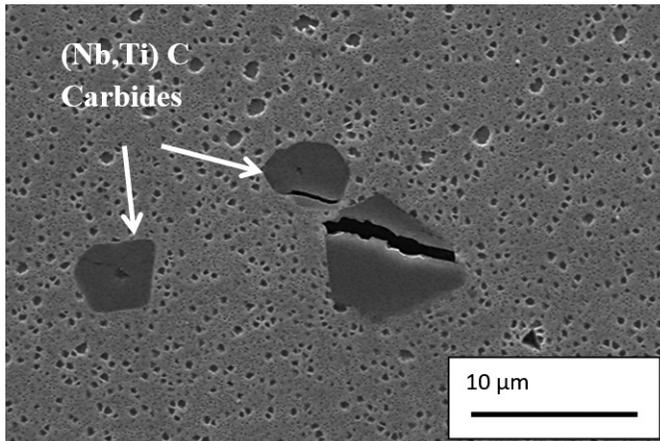
Figure 3. (f) Fatigue damage feature in the present alloy.
