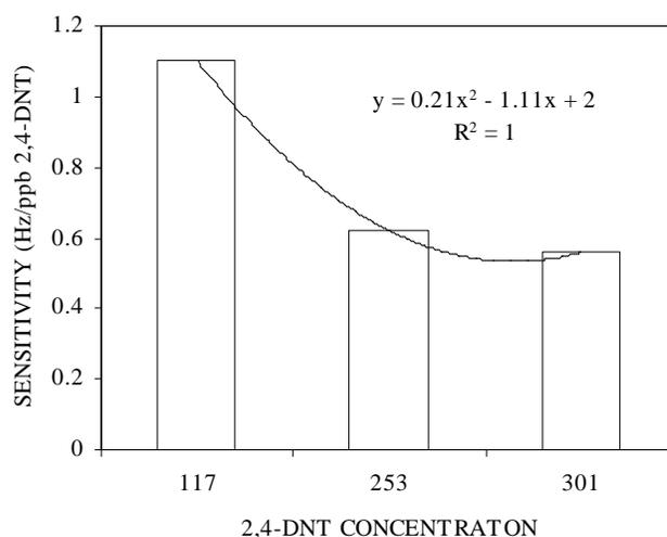
Figure 6. Typical linear response curve reported for the 2,4-DNT using 150 MHz SAW device.
