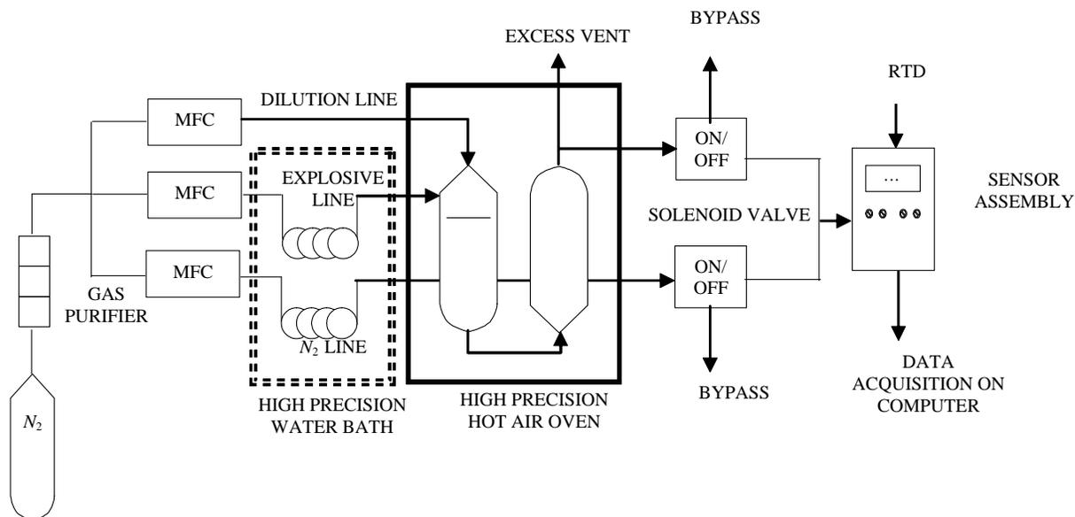
Figure 5. Schematic diagram of explosive vapour generation unit along with sensor calibration assembly<sup>30</sup>.
