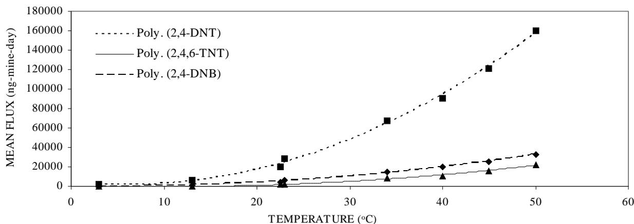
Figure 2. Mean flux into air for 2,4-DNB, 2,4-DNT, and 2,4,6-TNT from TMA5 landmines.
