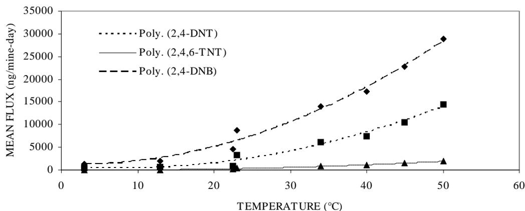
Figure 1. Mean flux into air for 2,4-DNB, 2,4-DNT, and 2,4,6-TNT from PMA1A landmines.
