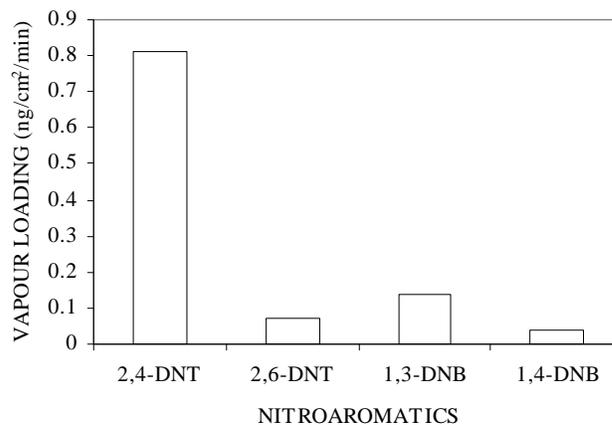
**Figure 7. A typical response of the carbowax polymer for various isomers and other nitroaromatic compounds reported.**
