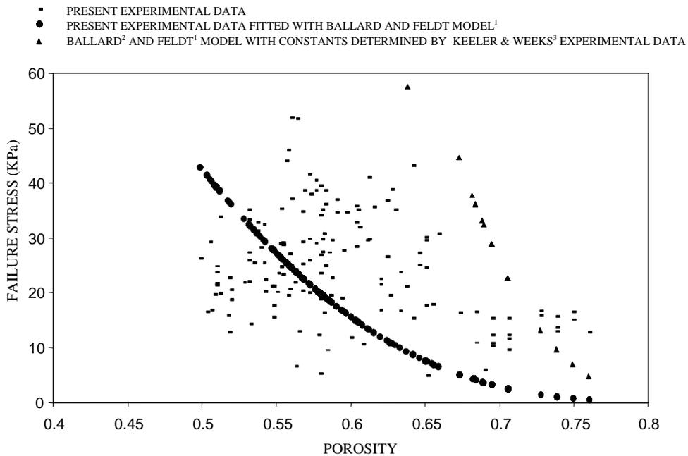
Figure 6. Comparison of experimental data with few porosity-dependent models.
