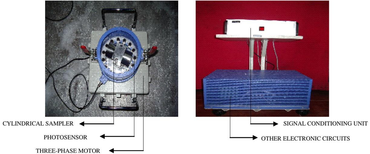
Figure 3. Experimental setup for centrifugal experiments in cold laboratory.
