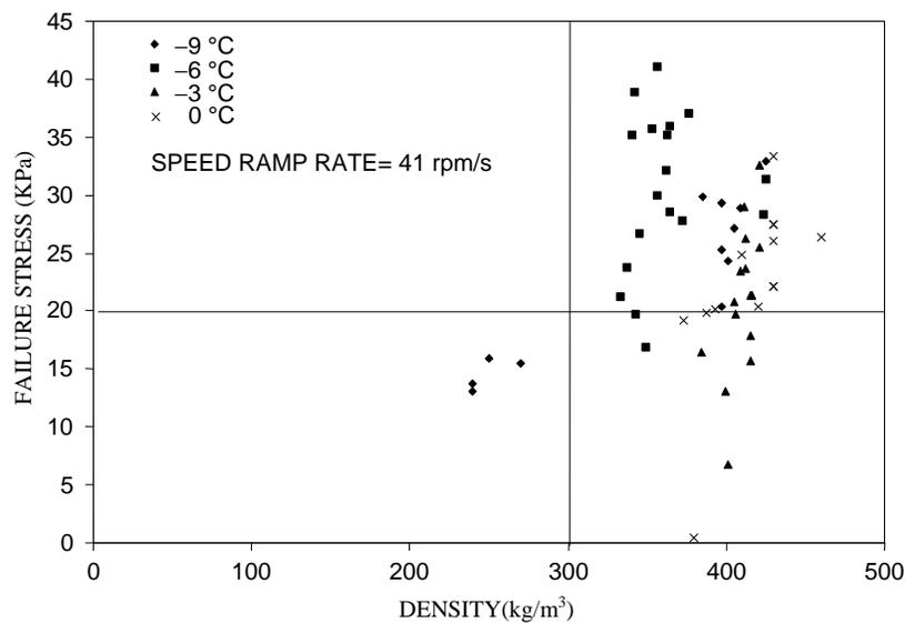
Figure 4. Dependence of tensile strength of snow on temperature and density for speed ramp rate of 41 rpm/s.
