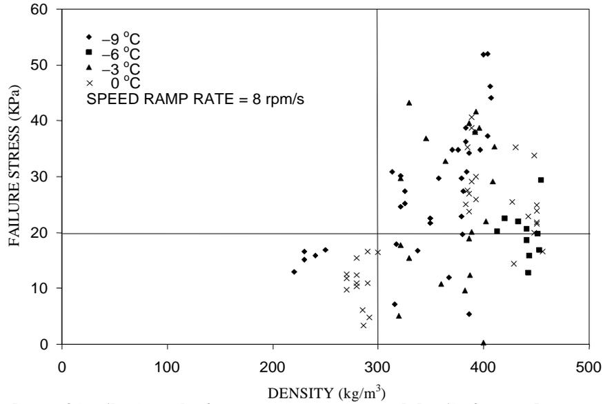
Figure 5. Dependence of tensile strength of snow on temperature and density for speed ramp rate of 8 rpm/s.
