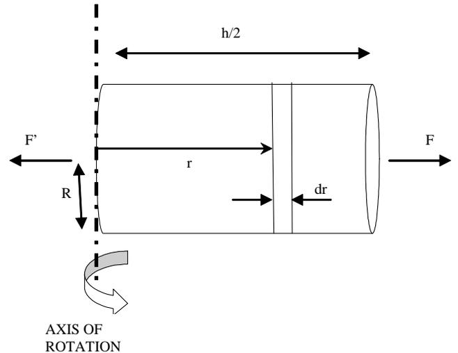
**Figure 1. Line diagram of snow sample under centrifugal loading.**
