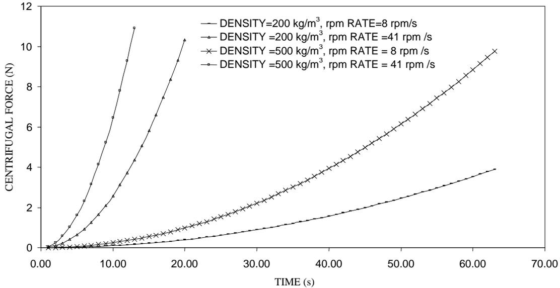
Figure 2. Dependence of input centrifugal force on sample density and ramp rate of rotation.
