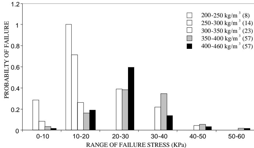
Figure 8. Probability distribution of tensile strength of snow in different density ranges.
