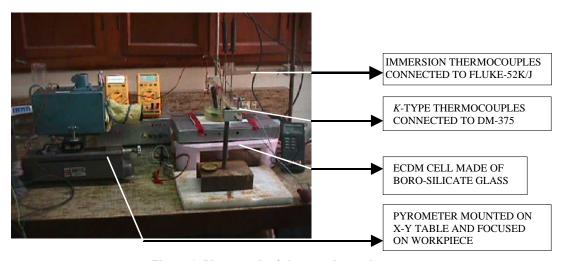
Figure 1. Photograph of the experimental set-up.
