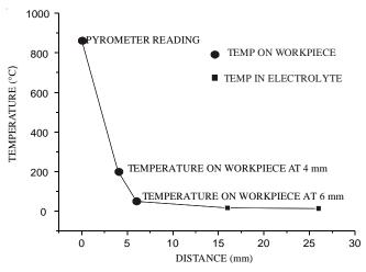
Figure 4. Experimentally measured temperature profile in ECDM.
