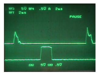
Figure 2. Synchronised time-varying current (upper waveform) and temperature (lower waveform) for copper workpiece<sup>16</sup>.
