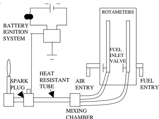
Figure 1. Schematic diagram of premixed flame test set-up.
