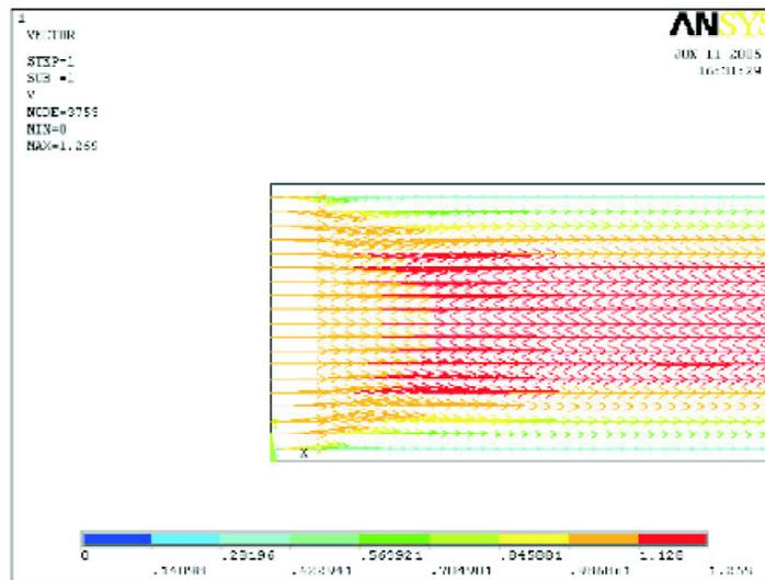
Figure 5. Velocity vectors at inlet of the duct.
