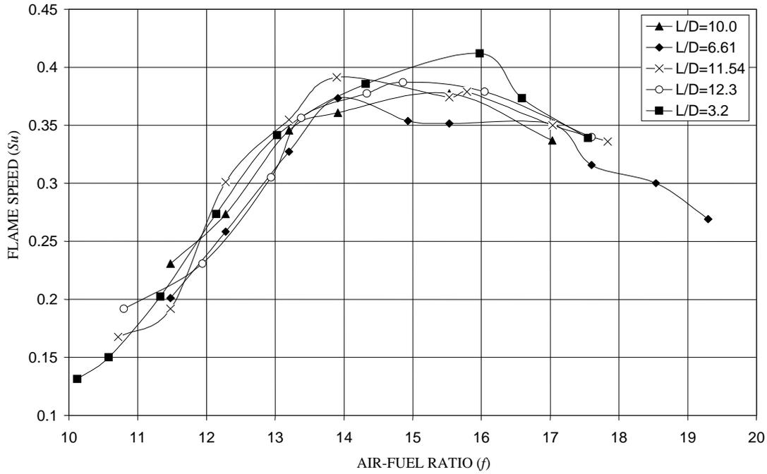
Figure 3. Variation of flame speeds with air-fuel ratio and different L/D ratios.
