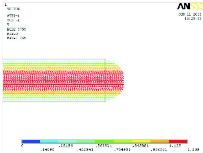
Figure 4. Velocity vectors for the mixture.
