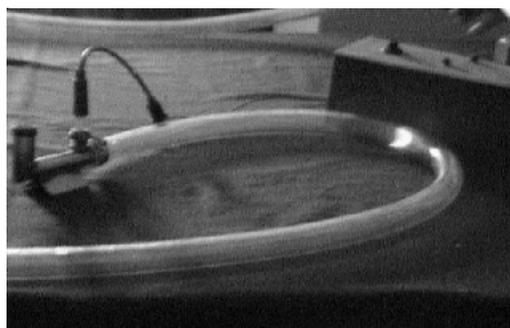
Figure 2. Premixed flame traveling in the heat-resistant tube of the test rig.
