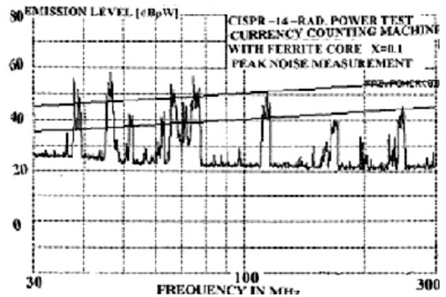
Figure 11. Peak Noise (dBpW) versus Frequency (MHz). Noise radiated by the currency counting machine (nickel-substituted *Li-Zn-Mn* Ferrite composition  $x=0.1$  used to suppress the electromagnetic noise).
