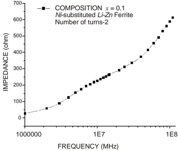
**Figure 3. Impedance versus frequency of Ni-substituted *Li-Zn* ferrite  $Li_{0.25-x/4}Zn_{0.5-x/2}Ni_xMn_{0.1}Fe_{2.15-x/4}O_4$  where  $x = 0.1$ .**
