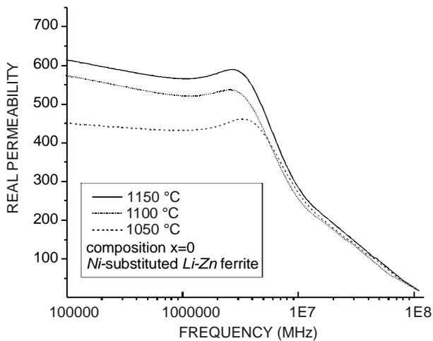
Figure 1. Real permeability ( $\mu'_s$ )/frequency of ferrite composition  $x=0$ ,  $Li_{0.25}Zn_{0.5}Mn_{0.1}Fe_{2.15}O_4$  ferrite material sintered at 1050 °C, 1100 °C, and 1150 °C.
