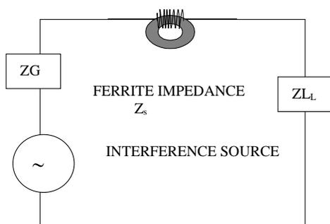
Figure 6. Application of ferrite core in the interference circuit.
