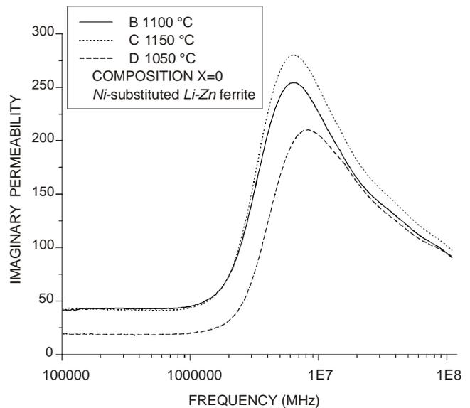
Figure 2. Imaginary permeability ( $\mu''_s$ )/frequency of ferrite composition  $x=0$ ,  $Li_{0.25}Zn_{0.5}Mn_{0.1}Fe_{2.15}O_4$  ferrite material sintered at 1050 °C, 1100 °C, and 1150 °C.
