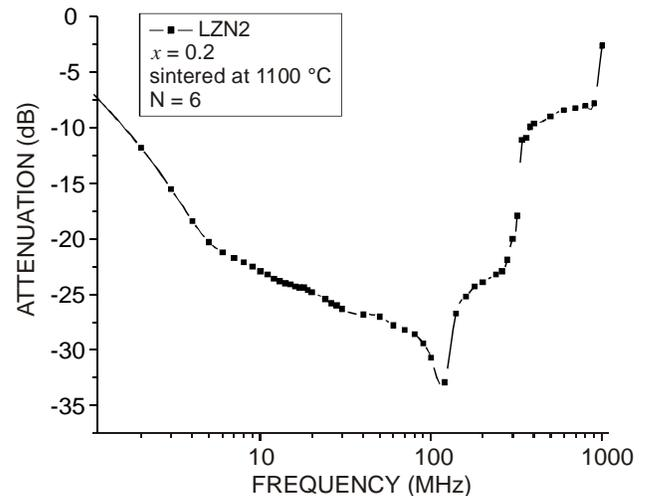
**Figure 5. Insertion loss versus frequency for the composition  $x = 0.2$ , number of turns  $n = 6$ .**
