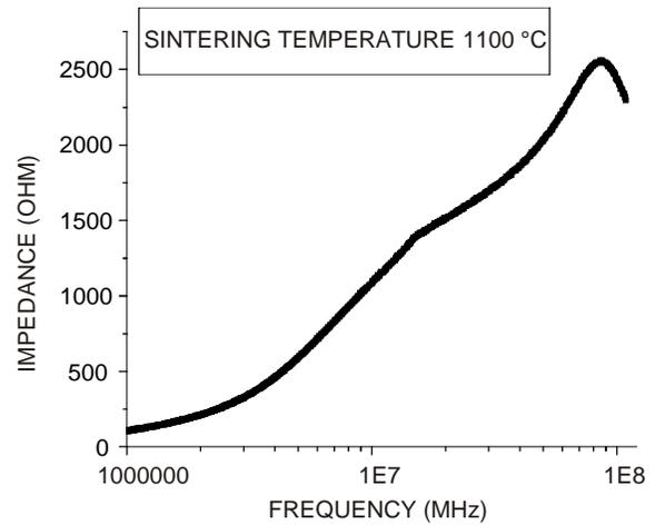
**Figure 4. Impedance versus frequency of Ni-substituted *Li-Zn* ferrite  $Li_{0.25-x/4}Zn_{0.5-x/2}Ni_xMn_{0.1}Fe_{2.15-x/4}O_4$  where  $x = 0.1$ .**
