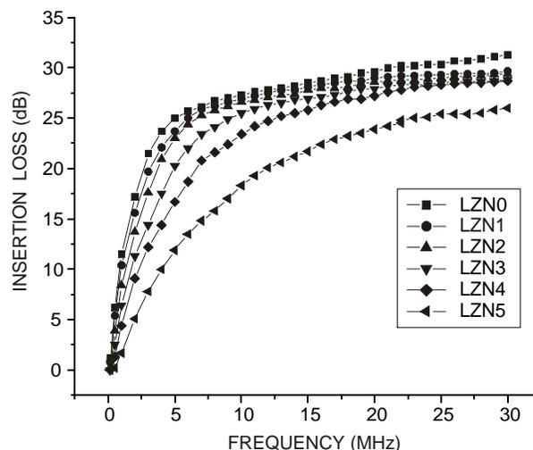
Figure 7. Insertion loss versus frequency (Mhz) for all the composition  $x=0$  to 0.5 (frequency range 1-30 MHz) number of turns  $N=6$ .
