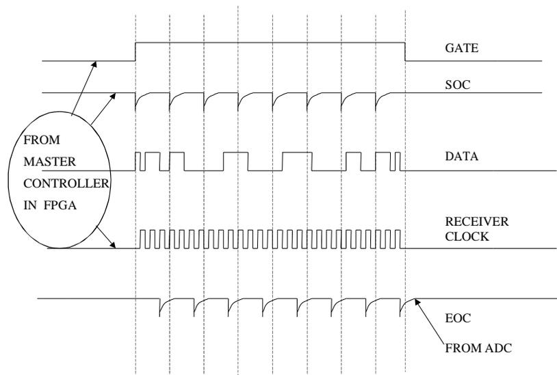
Figure 4. Control waveforms.
