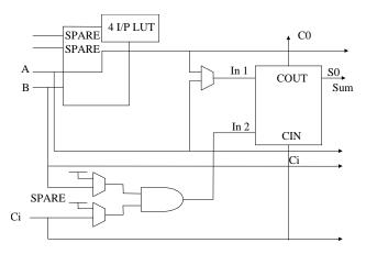
Figure 3. Basic FPGA cell.
