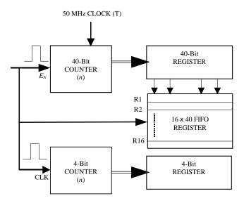
Figure 2. Block diagram of PRF-decoder.
