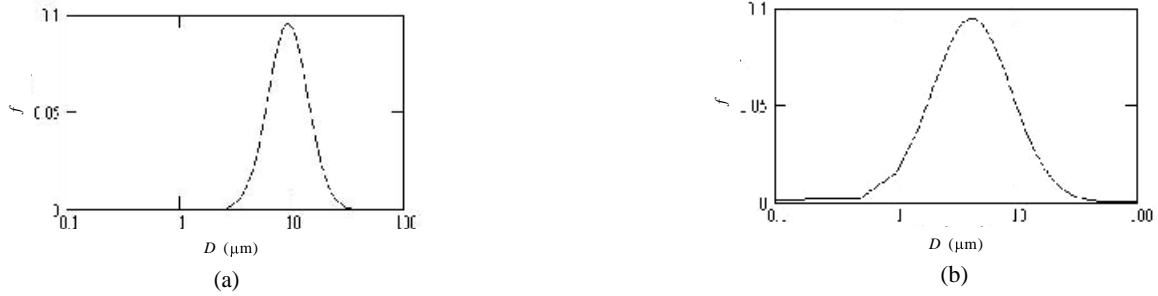
Figure 7. Density distribution of the particle diameter used in the calculation: (a) \sigma = 0.41 and \eta = 2.40 , and (b) \sigma = 0.75 and \eta = 2 .
