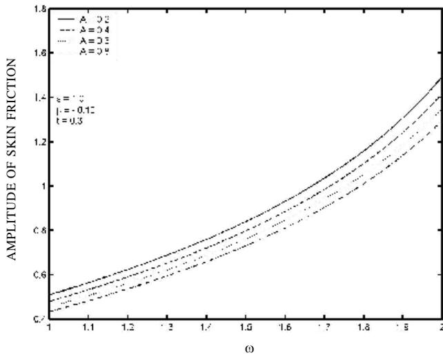
Figure 4. Effect of suction on the amplitude of skin friction.
