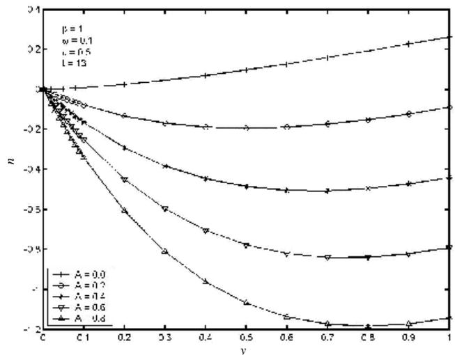
Figure 3. Velocity profiles for different values of suction parameter.
