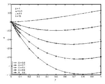
Figure 3. Velocity profiles for different values of suction parameter.
