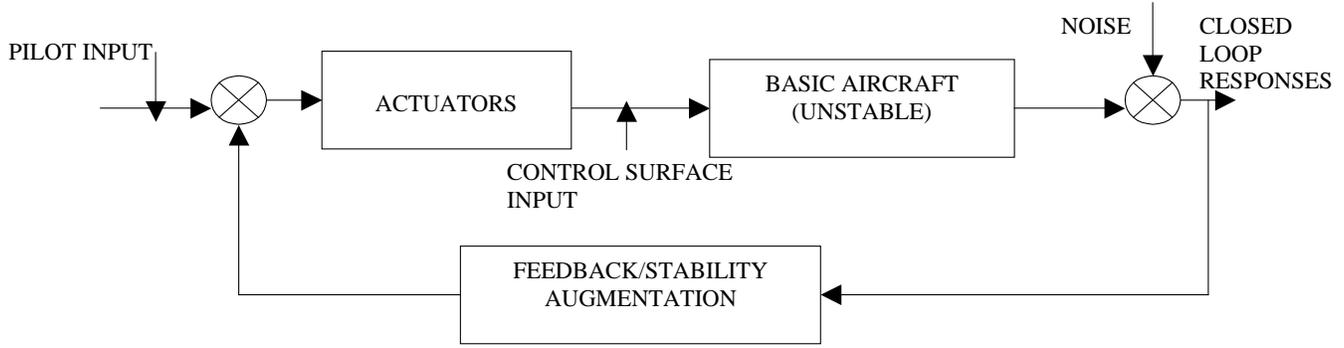
Figure 1. Block diagram of unstable/augmented aircraft.
