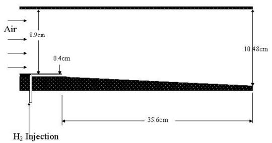
Figure 1. Experimental setup of Burrows and Kurkov<sup>10</sup>
