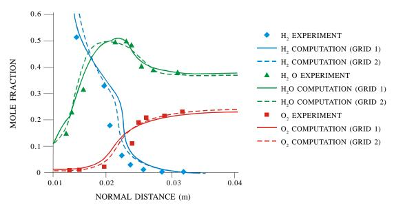
Figure 3. Comparison of computed results with experimental data for species mole fraction profiles at exit plane.
