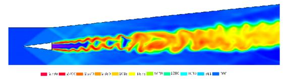
Figure 13. Field view of temperature.
