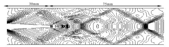
Figure 5. Pressure contours downstream of the strut.
