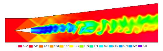
Figure 12. Mach number field view of combustion zone.
