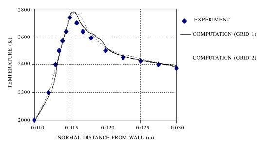
Figure 2. Comparison of predicted temperature in mixing layer at exit plane.
