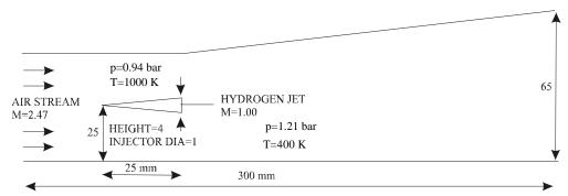
Figure 11. Schematic of the computational domain for strut injection.
