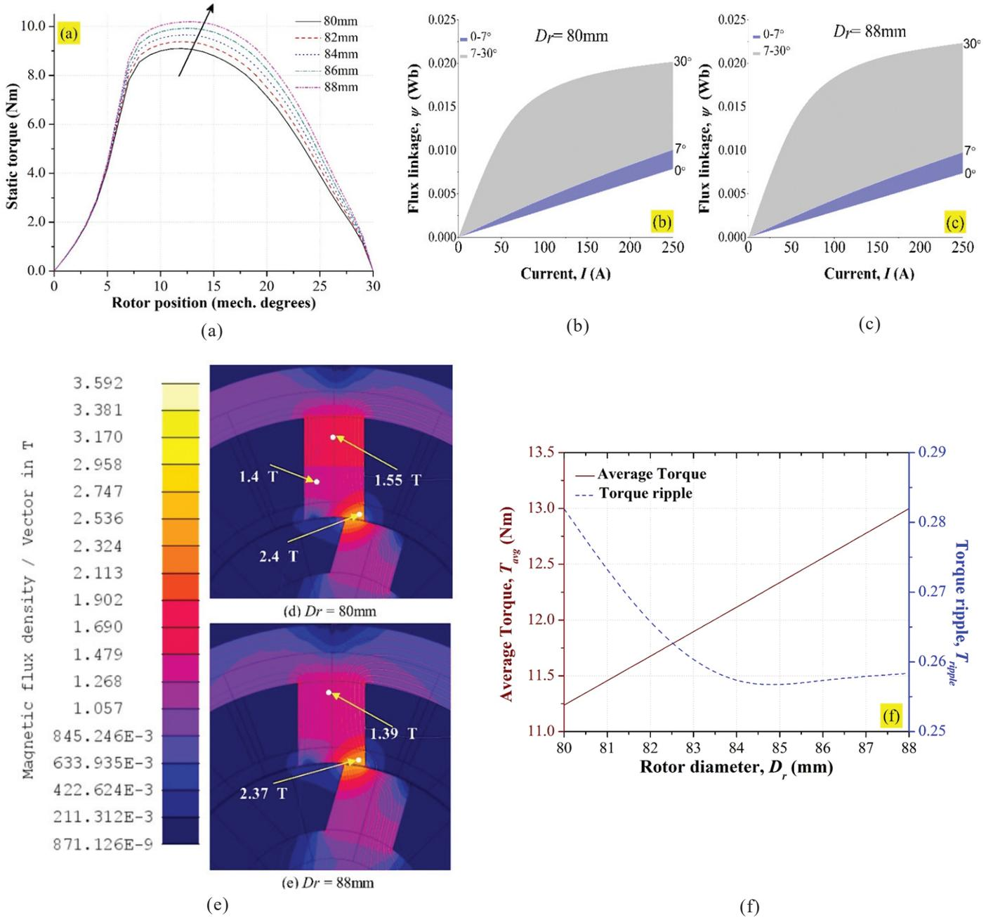
**Figure 3. Influence of change in  $D_r$ ; (a) Static torque profile, (b) and (c) Co-energy comparison between 80 and 88 mm designs (d) and (e) Flux density comparison (f) Average torque and torque ripple.**
