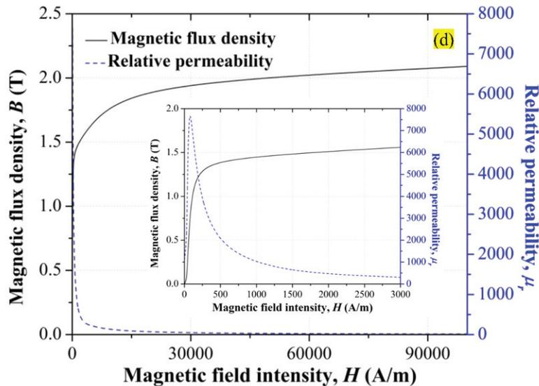
Figure 1. (a) Flux linkage vs current characteristics, (b) Flux path, (c) MEC for the flux path and (d) B-H curve of M270\_35A.
