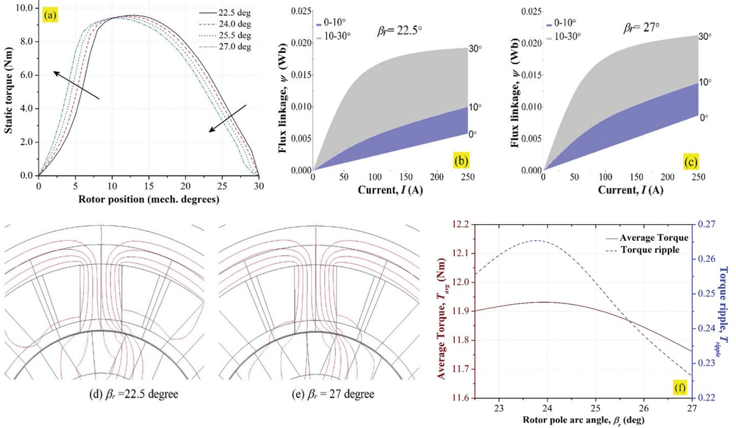
**Figure 5. Influence of change in  $\beta_r$ : (a) Static torque profile, (b) and (c) Co-energy comparison between 22.5 and 27 $^\circ$  designs, (d) and (e) Flux paths at 5 $^\circ$  rotor position and (f) Average torque and torque ripple.**
