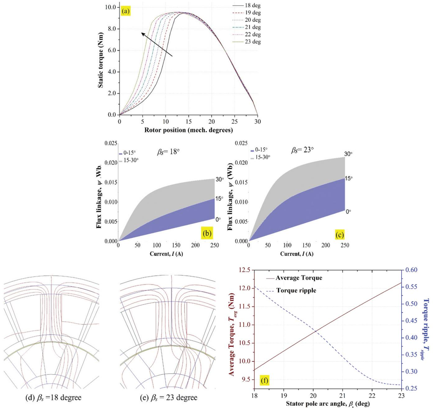
**Figure 4. Influence of change in  $\beta_s$ ; (a) Static torque profile, (b) and (c) Co-energy comparison between 18 and 23° designs (d) and (e) Flux paths at 8° rotor position (f) Average torque and torque ripple.**
