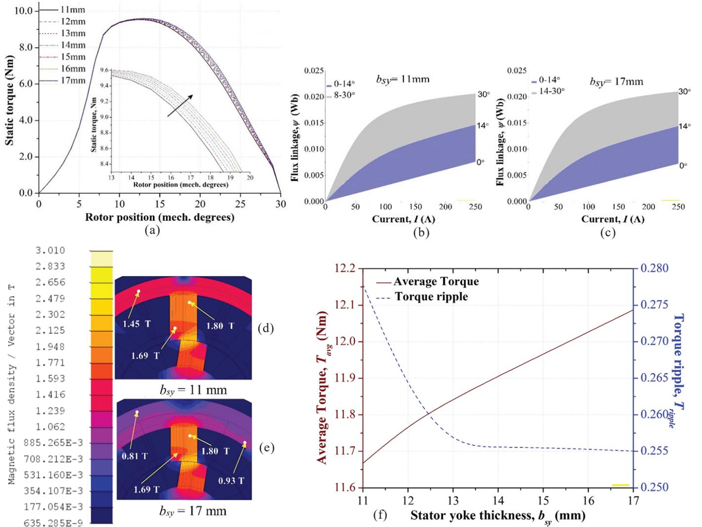
Figure 6. Influence of change in  $b_{sy}$ : (a) Static torque profile, (b) and (c) Co-energy comparison between 11 and 17 mm designs (d) and (e) Flux density comparison, (f) Average torque and torque ripple.
