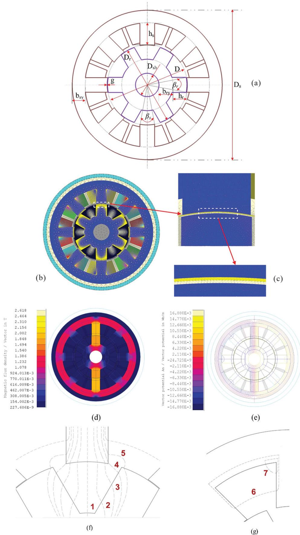
Figure 2. (a) Geometric design variables, (b) and (c) FEA model of the SRM, (d) Flux density plot, (e) Flux paths, (f) and (g) Flux paths at the unaligned position.
