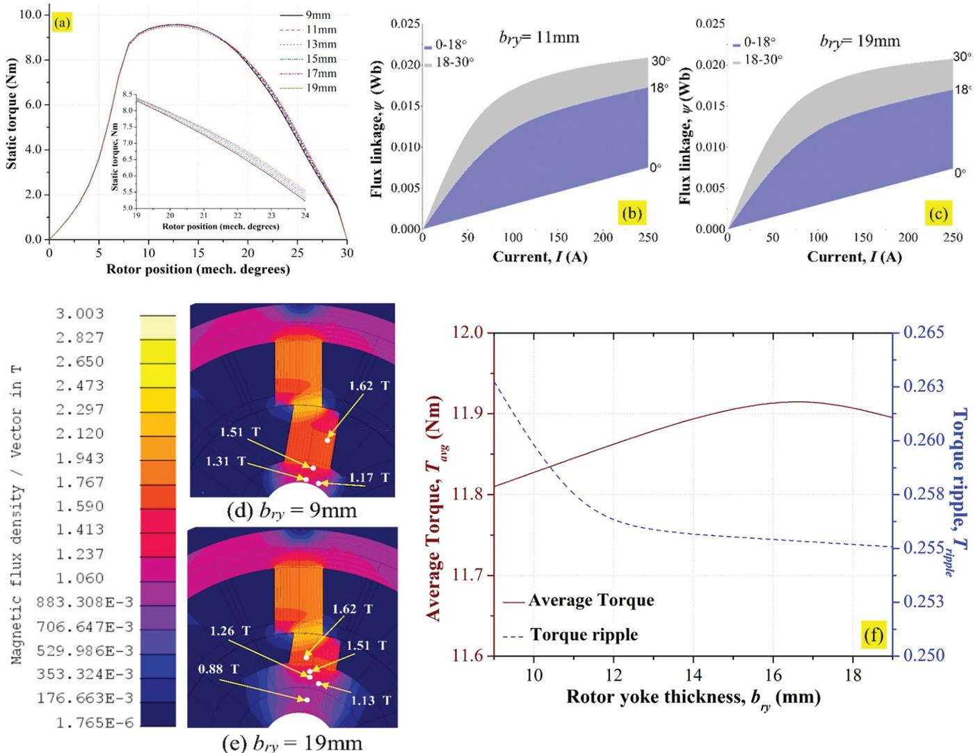
Figure 7. Influence of change in  $b_{ry}$ ; (a) Static torque profile, (b) and (c) Co-energy comparison between 9 and 19 mm designs (d) and (e) Flux density comparison (f) Average torque and torque ripple.
