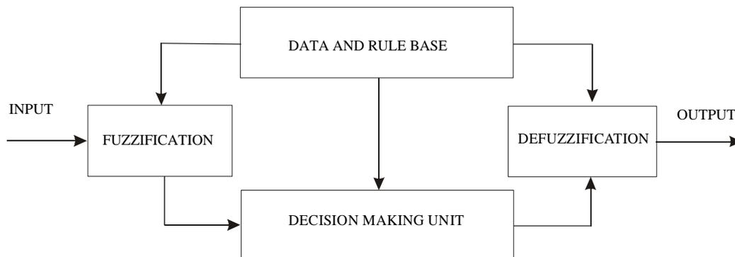
Figure 1. General structure of a fuzzy control system.
